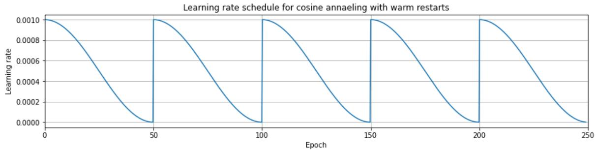
**Figure 5.4:** The learning rate following the cosine annealing with warm restarts schedule. Shown are 250 epochs with the schedule parameters being  $\eta_{min} = 10^{-7}$ ,  $\eta_{max} = 10^{-3}$ , and  $T_i = 50$ .
