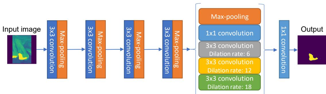
**Figure 5.14:** The DeepLab v3 architecture. A convolutional backbone processes images and Atrous Spatial Pyramid Pooling processes the resulting feature map. Next, the outputs of the ASPP module are concatenated and finally processed by a 1x1 convolution that produces the predicted segmentation mask.
