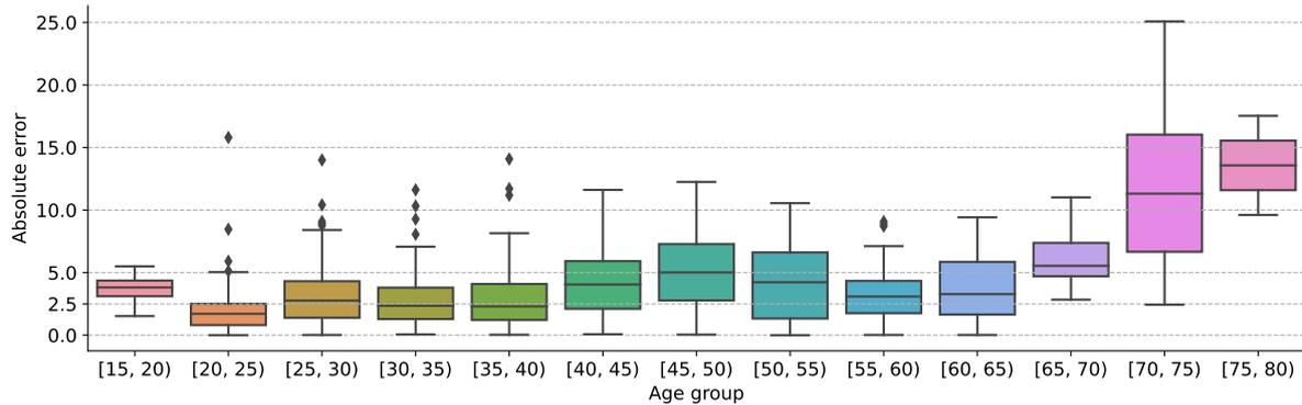
**Figure 6.5:** Overall results for age estimation with a probability distribution. As can be seen, the median absolute error across all age groups is lower compared to the direct regression approach, as is the variance of the error. Additionally, The absolute error does not consistently increase with age, as was the case with the direct regression approach.
