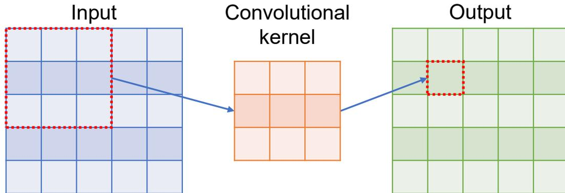
**Figure 2.2:** Visualization of how a tensor is processed by convolution. The convolution layer processes the input tensor with a sliding window, calculating the weighted sum as defined by its kernel for each position within it, thereby producing the output tensor.
