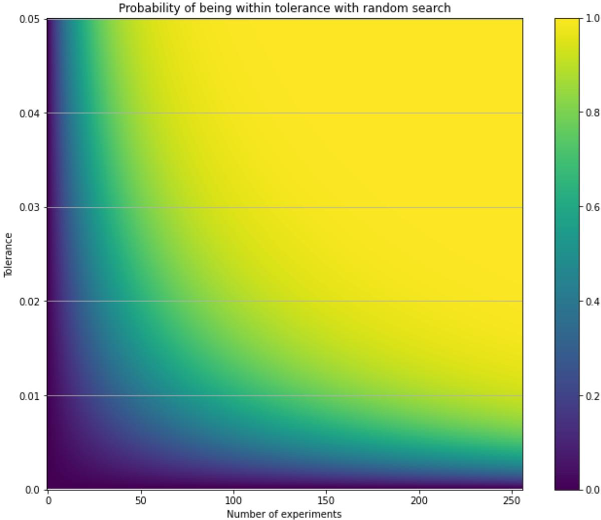
**Figure 5.2:** The probability map of a random search sample being within a tolerance per number of experiments. The x-axis represents the number of random samples (or the number of experiments for hyperparameter optimization), and the y-axis represents the tolerance from the global minimum in the restricted search space.
