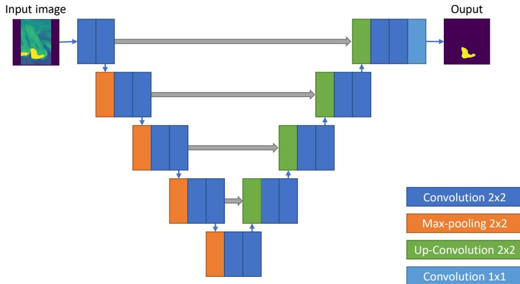
**Figure 5.15:** The baseline UNet architecture. An image is processed by a sequence of convolutions and max-pooling, after which it is upscaled using up-convolutions. Skip connections are added between the same scale in the "down" and "up" parts of the network. The network capacity is adjusted by changing the number of channels across all convolutional layers.
