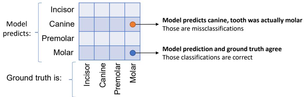
**Figure 5.9:** An example of a confusion matrix for a 4-class tooth type determination model. The rows represent the model predictions, and the columns represent the ground truth values. The figure shows an example of a correct classification (molar-molar) and a misclassification (canine-molar).
