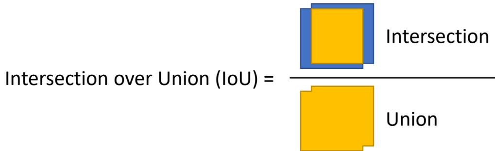
**Figure 5.16:** The Jaccard index, also called the Intersection over Union. The metric describes the percentage of overlap between the ground truth and predicted regions, thus avoiding the true negative bias of the per-pixel accuracy.
