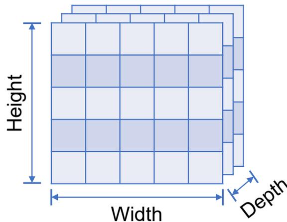
**Figure 2.1:** A representation of a 3D tensor. A 3D tensor can be imagined as a stack of 2D images of the same width and height. The number of images in this stack is the depth of the tensor, which can also be described as *the number of channels*. In computer vision, a tensor of this shape is sometimes called a *feature map*.
