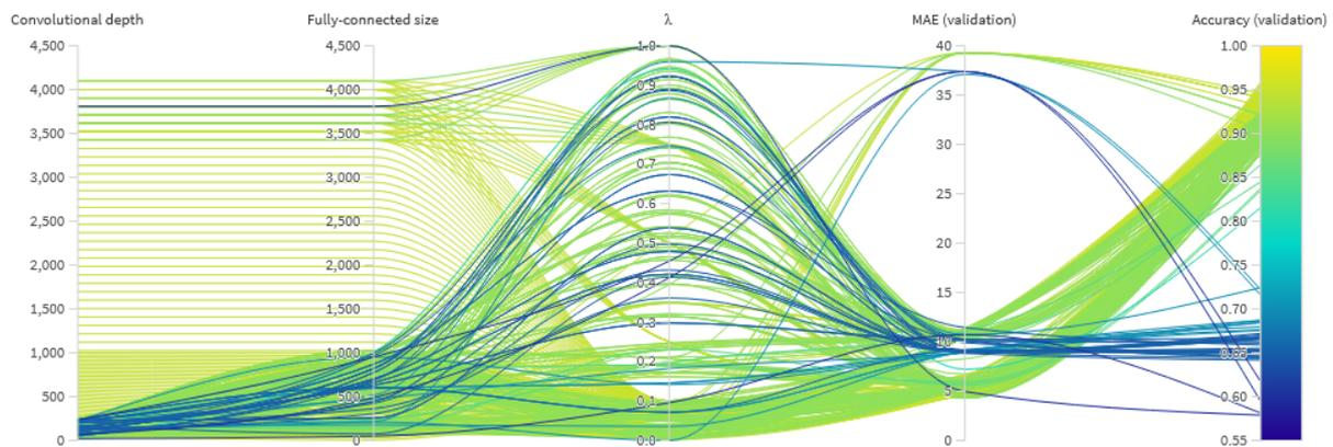
**Figure 5.10:** Parallel coordinates plot of grid and random search for multi-task models that simultaneously estimate age and assess sex. Grid and random search initially used a range for  $\lambda$  between 0 and 1. On the second iteration of hyperparameter optimization, the range was reduced between 0 and 0.1, as that interval performed best.
