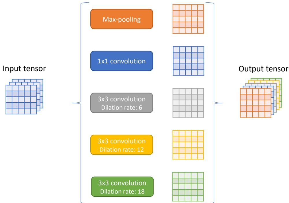
**Figure 5.13:** Visualization of Atrous Spatial Pyramid Pooling. The same feature map is processed at different scales using atrous convolutions. This produces feature maps of the same size, but due to the dilation factor, the processing is effectively on different scales.
