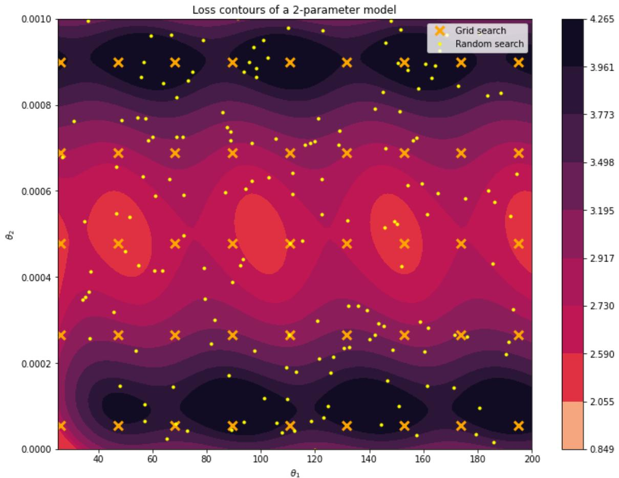
**Figure 5.3:** Visualization of grid and random search samples on a contour plot of a loss function for a 2-parameter model. The orange X shows points sampled by grid search, while the yellow dots show points sampled by random search. As can be seen, both methods manage to sample points close to the minima.
