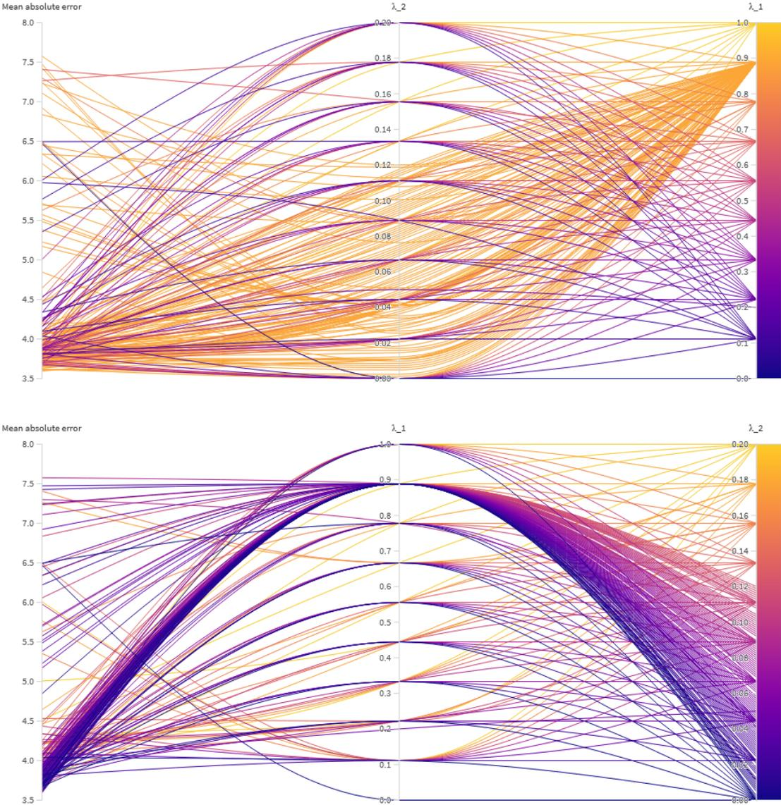
**Figure 6.6:** The effect of the  $\lambda$  values on the mean absolute error. The mean absolute error is the leftmost axis. The upper figure is colored according to the value of  $\lambda_1$ , and the lower by the value of  $\lambda_2$ .
