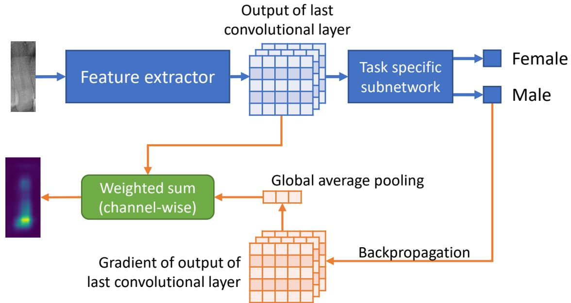
**Figure 2.3:** GradCAM uses the gradient of the output of the feature extractor to calculate the saliency map for interpretability. Global average pooling is used to calculate the gradient-based weight vector. The resulting saliency map is the weighted sum (channel-wise) of the last convolution layer's feature map and the gradient-based weight vector.
