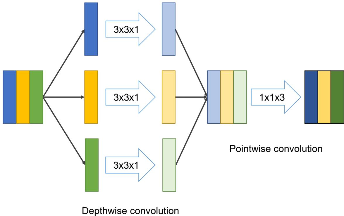
**Figure 4.3:** Overview of a 3x3 depthwise separated convolution on a 3-channel tensor. The convolution is split into two operations that apply two smaller kernels, which results in a net decrease in parameters. The trade-off is a slight increase in computation time.
