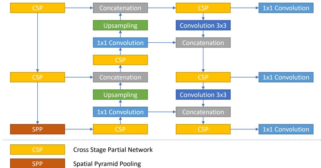
**Figure 5.17:** The architecture of the YOLO v5 detection model. The architecture uses multiple CSP modules and a high degree of skip connections and concatenations to allow for easier gradient calculations.
