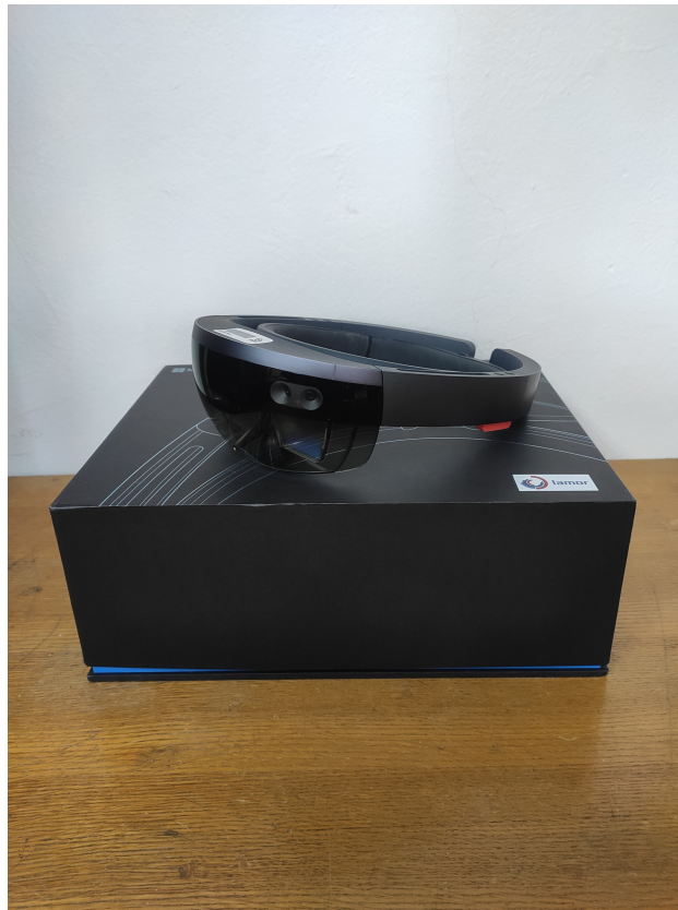
Figure 2.3: The Microsoft HoloLens 2.0 Development Edition augmented reality glasses are used for several experiments in the scope of this thesis.
