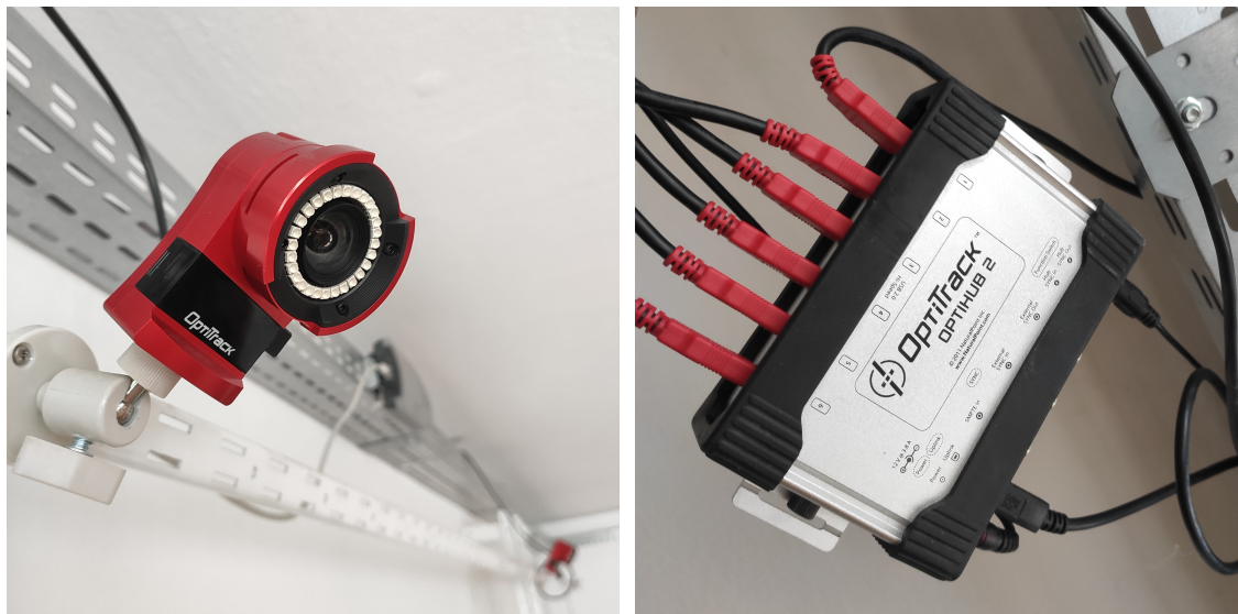
(a) One of twelve Flex 13 motion capture cameras used for dataset recording. (b) The OptiHub 2 - a USB hub connected to cameras, the other hub, and a PC collecting and broadcasting recorded data.
