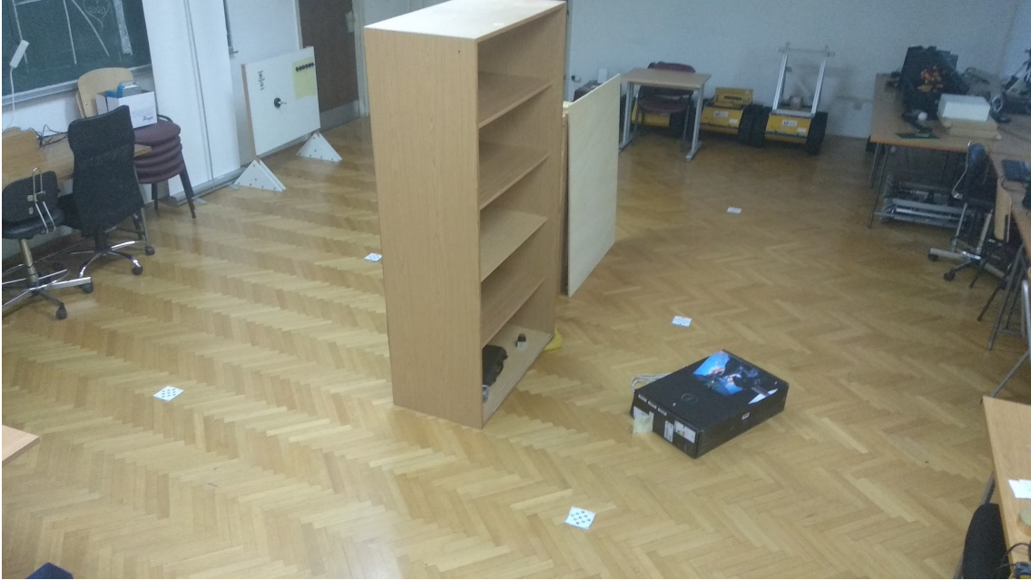
Figure 5.7: A setup for localization experiments with moving UWB anchors. Two moving UWB anchors are placed on the boxes which simulate moving robots.
