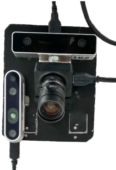
Figure 2.8: RealSense D435 camera placed in between viewing areas of stereo camera and monocular camera to improve extrinsic calibration. Only a color camera was used during the calibration.
