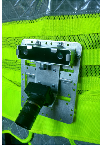
Figure 2.6: Safety Vest with the sensor setup that consists of an IMU-aided stereo camera and a downward-looking monocular camera. This placement of the sensors was chosen since it will not disturb the human when performing the usual tasks. Furthermore, cameras cannot get obstructed by hands, and this part of the human body is the most stable and has the smallest chance of doing abrupt motion that could blur the images.
