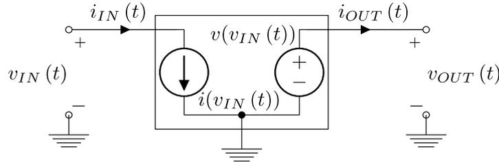
**Figure 3.1:** The basic interchangeable behavioural model architecture [36].
