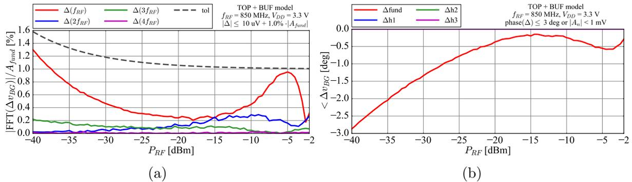
**Figure 3.11:** Behavioural model accuracy evaluation in the top-level test bench with the BUF behavioural model under an RF forward power sweep at 850 MHz: (a) relative amplitude error in percent, (b) phase error per harmonic component, with the tolerance limit of  $3^\circ$ .
