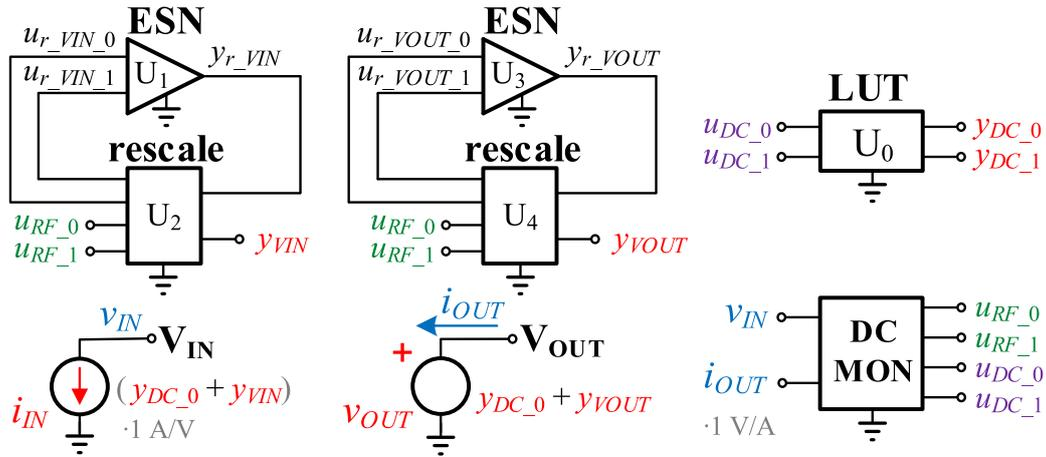
**Figure A.1:** The behavioural model of a generic 2-port circuit block. The input current  $i_{IN}$  and output voltage  $v_{OUT}$  are modelled as functions of the input voltage  $v_{IN}$  and output current  $i_{OUT}$ .
