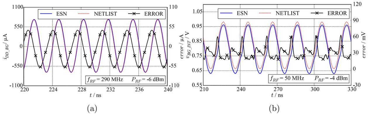
**Figure 3.26:** The reference and modelled time-domain waveforms of the modelled BG subcircuit and the instantaneous model error, taken at the worst-case MSE points: (a) input current model, (b) output voltage model [36].
