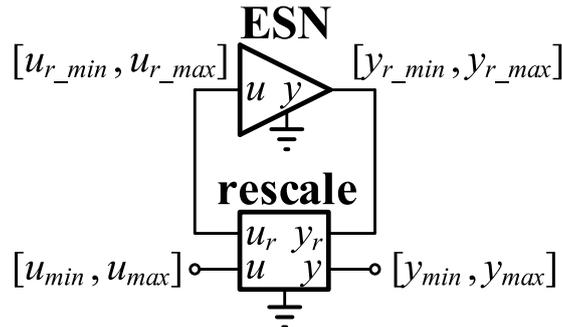
**Figure 2.5:** Echo state network with the rescaling block.
