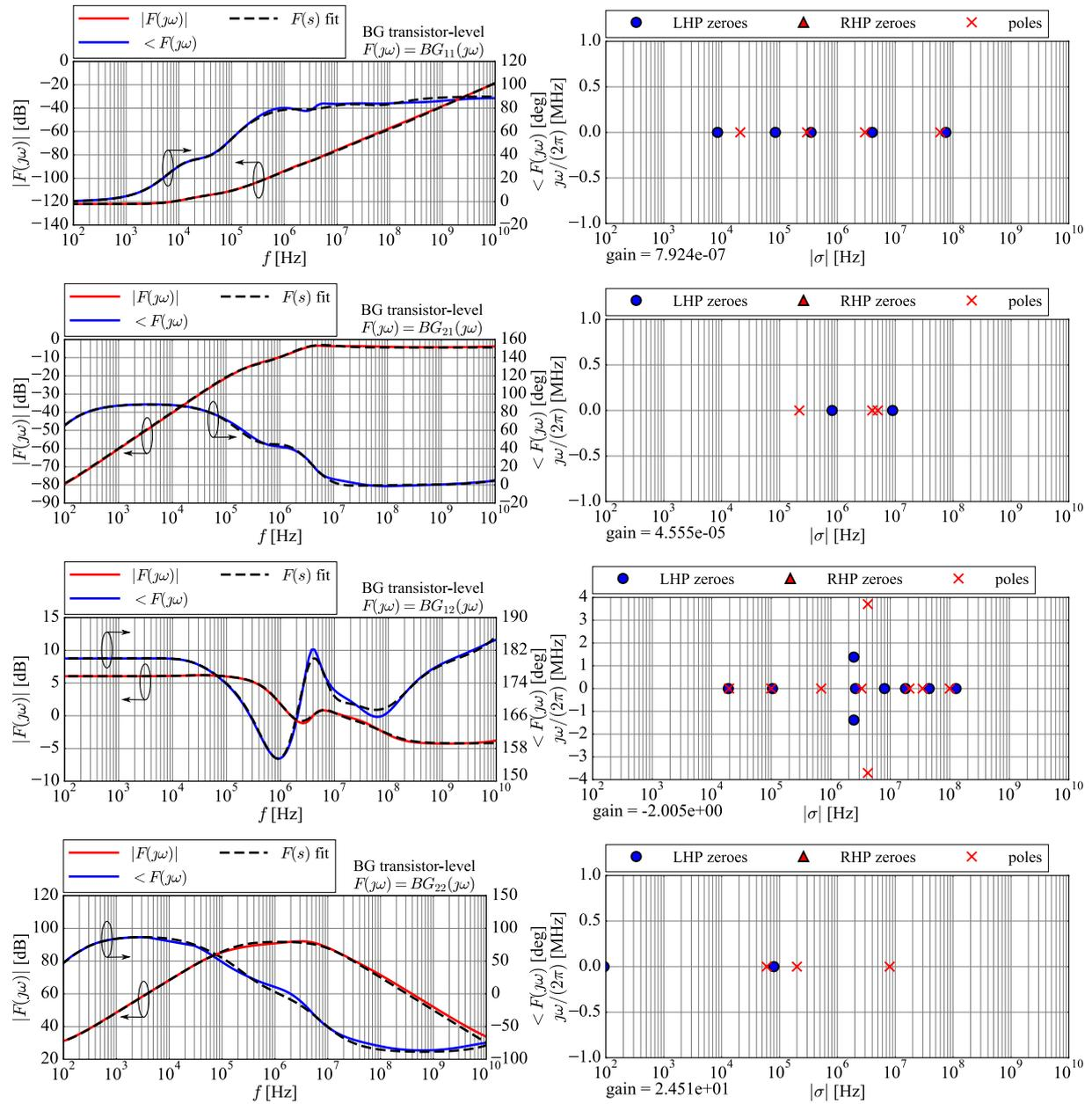
**Figure B.11:** Frequency responses  $BG_{ij}(j\omega)$  of the transistor-level bandgap block (solid lines), with the associated transfer functions  $BG_{ij}(s)$  in the  $s$ -domain, where  $s = 2\pi\sigma \pm j\omega$ .
