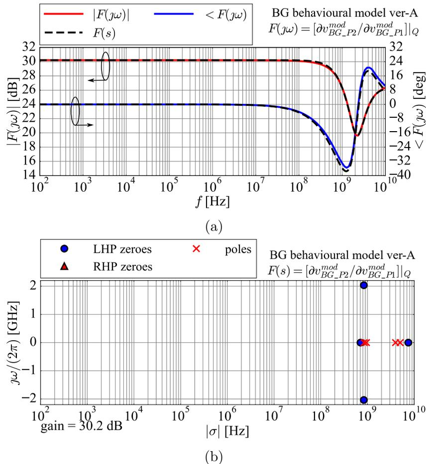
**Figure 3.19:** (a) Frequency response  $BG_{mod\_21}(j\omega)$  of the transfer function from the supply voltage  $v_{BG\_P1}$  to the output voltage  $v_{BG\_P2}$  of the BG behavioural model instance ver-A, obtained by simulations (solid lines), and the frequency response of the fitted transfer function with the poles and zeroes shown in (b) (dashed lines), (b) positions of the 4 poles and 4 zeroes in the LHP of the  $s$ -domain of the analytical small-signal model  $BG_{mod\_21}(s)$  [38].
