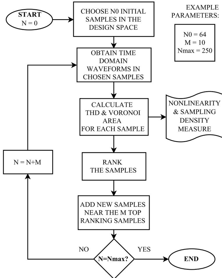
**Figure 2.6:** Flow chart of the proposed adaptive algorithm for sampling the nonlinear circuit behaviour in the time-domain [37].
