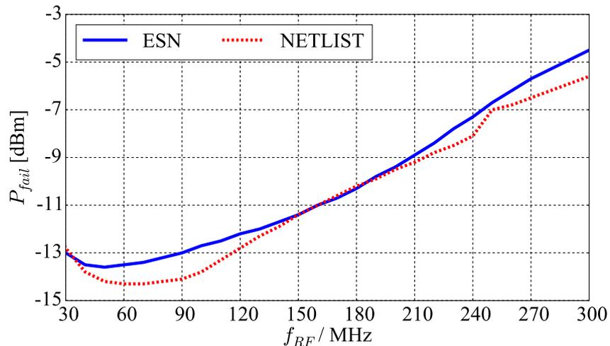
**Figure 3.27:** The comparison between the DPI characteristics of the DUT obtained using the time-domain simulations of the behavioural model (dotted line) and the transistor-level model (solid line) of the BG circuit [36].
