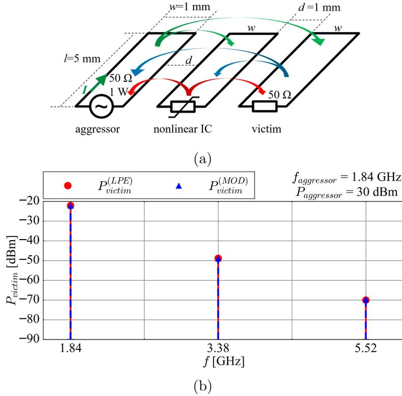
**Figure 4.8:** (a) Measurement setup for IC pin nonlinearity characterization based on the diplexer (DPLX) [66], [67], including the RF signal generator (SG), spectrum analyzer (SA), and test board (PCB), (b) PSS simulation of the wireless system test case where the aggressor operates at 1.84 GHz and the available power of 1 W = 30 dBm [45].
