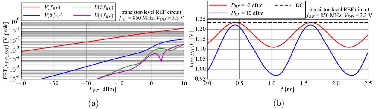
**Figure 3.8:** RF forward power sweep simulation of the transistor-level REF circuit in the top-level test bench from -40 dBm to 10 dBm at a constant RF frequency of 850 MHz of the BG output voltage  $v_{BG\_INT}$ : (a) harmonic components as a function of RF forward power  $P_{RF}$ , (b) time-domain waveforms at the RF forward power levels of -2 dBm and 10 dBm, with the DC operating point value of  $V_{BG\_INT} = 1.23381$  V [38].
