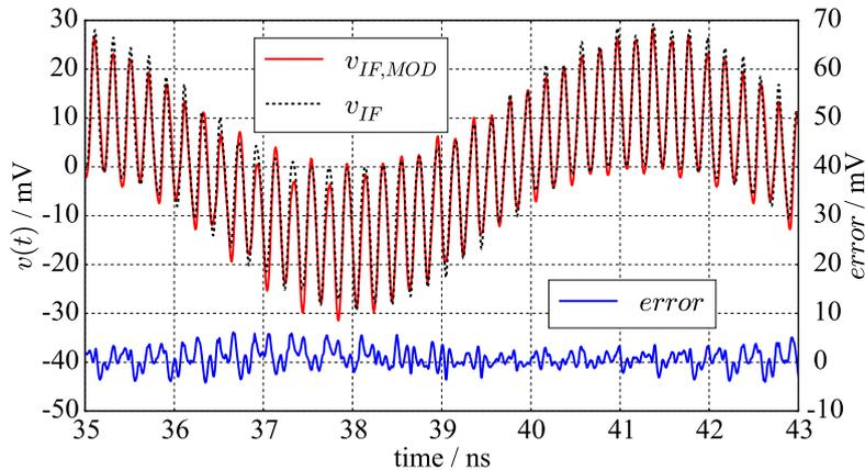
**Figure 2.18:** Performance of the ESN model compared with the reference output signal for the case with  $f_{IF,LOW} = 150$  MHz,  $f_{RF} = 2.40$  GHz,  $f_{LO} = 2.55$  GHz,  $f_{IF,HIGH} = 4.95$  GHz,  $error = v_{IF} - v_{IF,MOD}$  [34].
