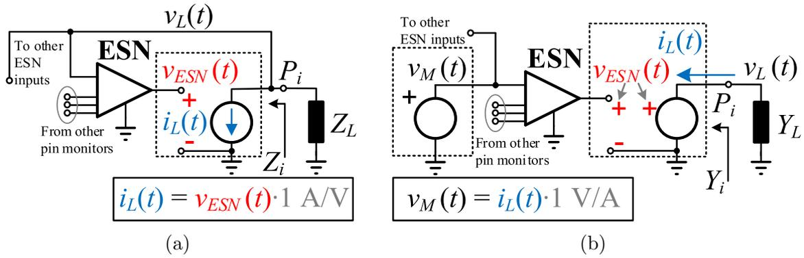
**Figure 3.2:** Dual nonlinear impedance behavioural models based on the echo state network (ESN) with a feedback loop: (a) monitoring voltage  $v_L(t)$  and driving current  $i_L(t)$ , (b) monitoring current  $i_L(t)$  and driving voltage  $v_L(t)$  [38].
