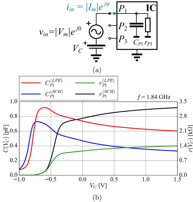
**Figure 4.6:** (a) Simulation testbench used for extracting the values of the capacitance  $C_{P1}$  and dynamic resistance  $r_{P1}$  as a function of the bias voltage  $V_C$ , according to [69], (b) voltage-dependent RC term values of the IC pin  $P_1$ , extracted from simulations of the schematic netlist (*SCH*), and the netlist including layout parasitic elements (*LPE*) [45].
