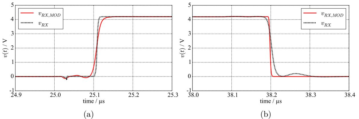
**Figure 2.15:** ESN model output compared to the reference output signal: (a) rising edge of the modelled signal, (b) falling edge of the modelled signal. The mean square error is  $1.771 \cdot 10^{-3}$  [34].
