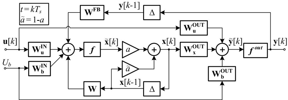
**Figure 2.2:** The signal flow-diagram of the echo state network as a discrete-time system with the constant sampling time  $T_s$  and the leaky integrator neuron model defined by the leaking rate  $a$ .
