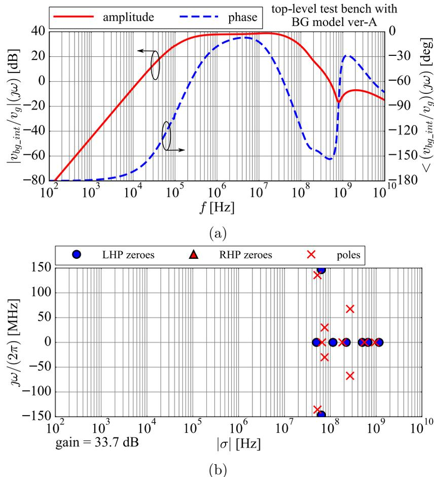
**Figure 3.20:** (a) Frequency response associated with the closed-form solution of the voltage perturbation  $v_{bg\_int}$  versus the RF generator  $v_g$  in the top-level test bench with the BG behavioural model instance ver-A, (b) analytical small-signal model fitted to the frequency response, with 12 poles and 12 zeroes in the LHP of the  $s$ -domain [38].
