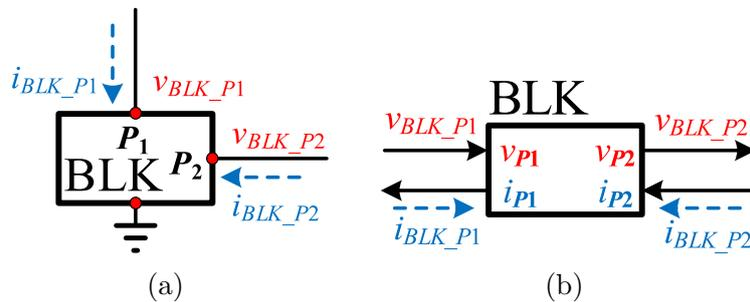
**Figure 3.3:** Definition of a generic 2-port circuit: (a) circuit schematic, (b) signal flow-diagram. The port voltages are referenced to the ground pin, and the port current direction is indicated by dashed arrows. The solid arrows in (b) indicate if a voltage or current is an input or an output signal [38].
