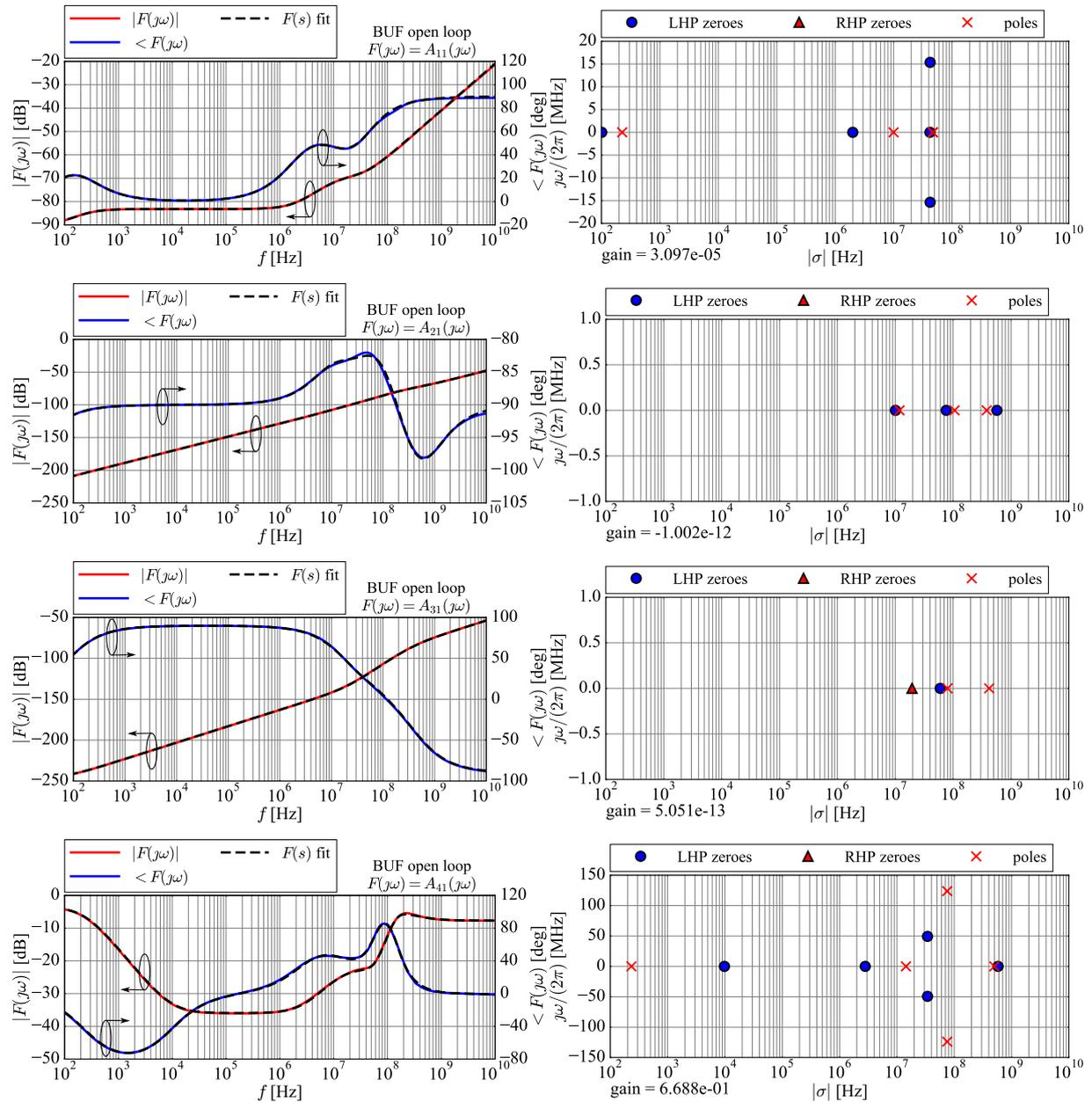
**Figure B.4:** Frequency responses  $A_{i1}(j\omega)$  of the transistor-level output buffer in the open loop (solid lines), with the associated transfer functions  $A_{i1}(s)$  in the  $s$ -domain against the input voltage  $v_1$ , where  $s = 2\pi\sigma \pm j\omega$ .
