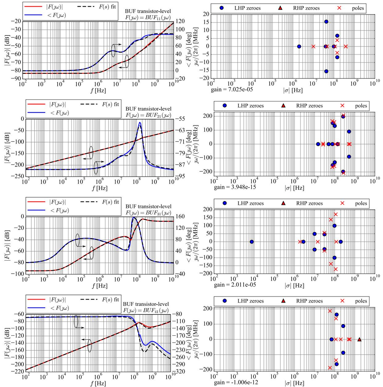
**Figure B.8:** Frequency responses  $BUF_{i1}(j\omega)$  of the transistor-level output buffer in the voltage follower configuration (solid lines), with the associated transfer functions  $BUF_{i1}(s)$  in the  $s$ -domain against the input voltage  $v_{P1}$ , where  $s = 2\pi\sigma \pm j\omega$ .
