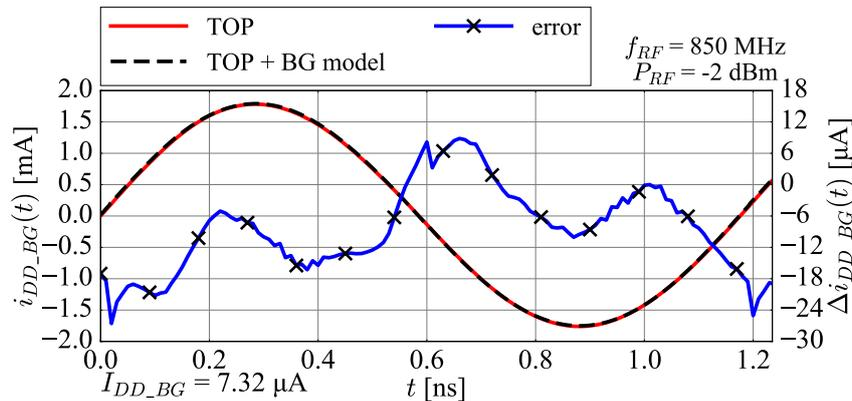
**Figure 3.28:** Comparison of time-domain waveforms of the BG supply current  $i_{DD\_BG}(t)$  at  $P_{RF} = -2$  dBm in the top-level test bench with the BG behavioural model, where the highest relative mean value error of 120% is observed. The amplitude of 1.8 mA is 245 times higher than the reference DC value  $I_{DD\_BG}$  of 7.32  $\mu\text{A}$ , and small errors of the time-domain samples near the peak result in a large relative error of the mean value [38].
