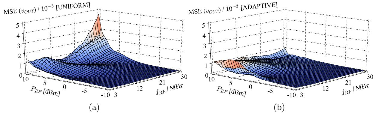
**Figure 2.10:** MSE of the  $v_{OUT}$  model of the voltage follower built using: (a) uniform sampling, with  $MSE_{\max} = 4.59 \cdot 10^{-3}$ , (b) adaptive sampling, with  $MSE_{\max} = 1.60 \cdot 10^{-3}$  [37].
