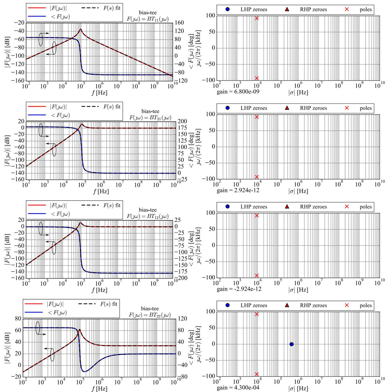
**Figure B.13:** Frequency responses  $BT_{ij}(j\omega)$  of the bias-tee with a 50- $\Omega$  RF generator (solid lines), with the associated transfer functions  $BT_{ij}(s)$  in the  $s$ -domain, where  $s = 2\pi\sigma \pm j\omega$ .
