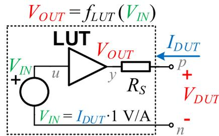
**Figure 4.3:** Architecture of the behavioural model of the ESD protection device TLP characteristic based on [62]. The look-up table (LUT) is built from the TLP measurement data [44].
