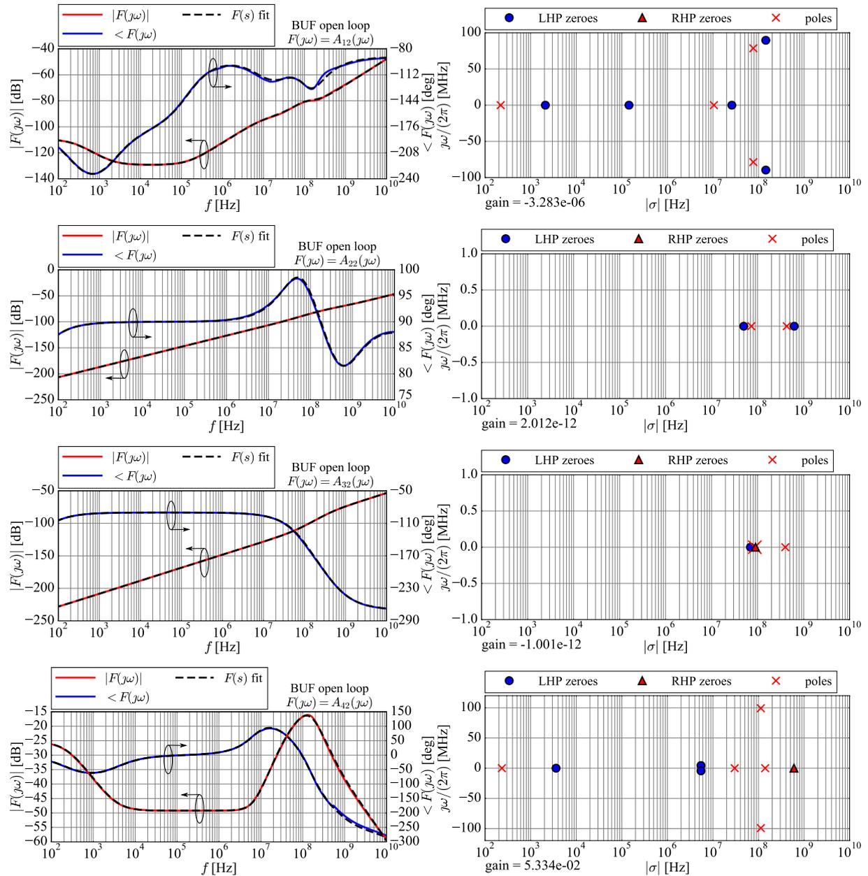
**Figure B.5:** Frequency responses  $A_{i2}(j\omega)$  of the transistor-level output buffer in the open loop (solid lines), with the associated transfer functions  $A_{i2}(s)$  in the  $s$ -domain against the common-mode input voltage  $v_{2C}$ , where  $s = 2\pi\sigma \pm j\omega$ .
