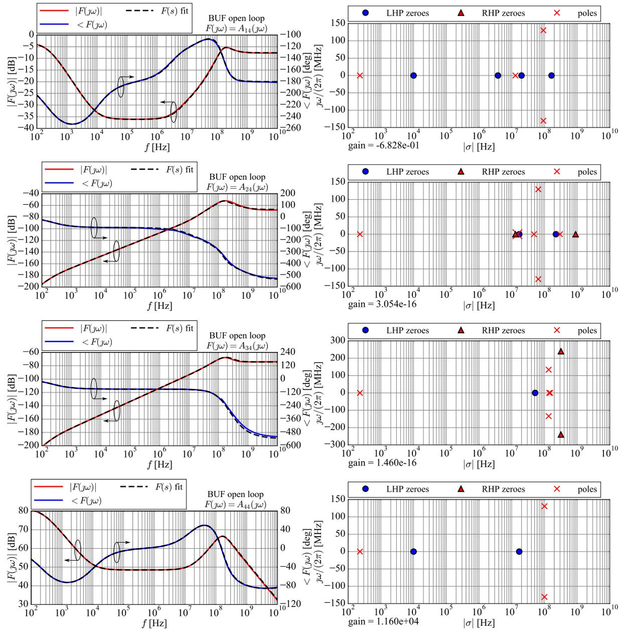
**Figure B.7:** Frequency responses  $A_{i4}(j\omega)$  of the transistor-level output buffer in the open loop (solid lines), with the associated transfer functions  $A_{i4}(s)$  in the  $s$ -domain against the output current  $i_3$ , where  $s = 2\pi\sigma \pm j\omega$ .
