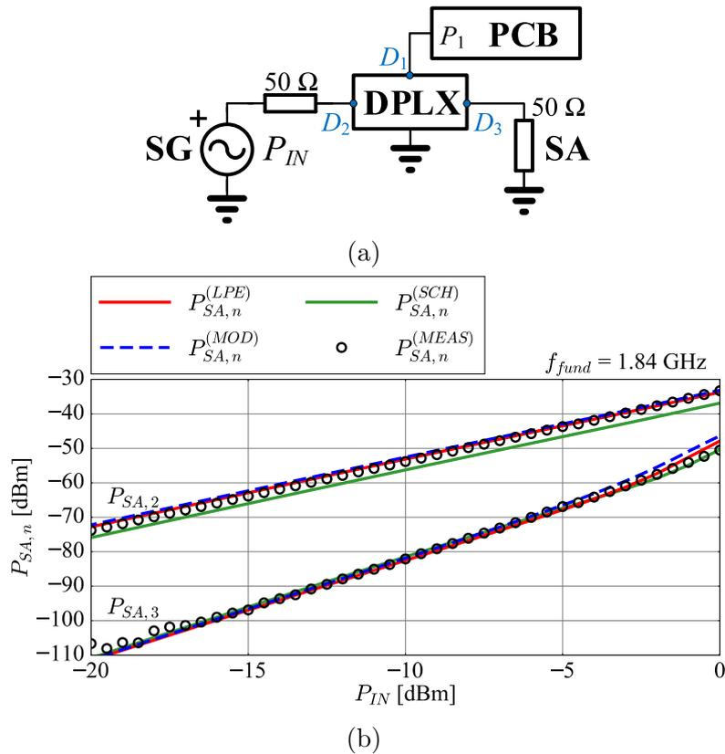
**Figure 4.7:** (a) Measurement setup for IC pin nonlinearity characterization based on the diplexer (DPLX) [66], [67], including the RF signal generator (SG), spectrum analyzer (SA), and test board (PCB), (b) comparison between measurement and behavioural model simulation of the power at second harmonic  $P_{SA,2}$  and third harmonic  $P_{SA,3}$  in the diplexer setup at 1.84 GHz [45].
