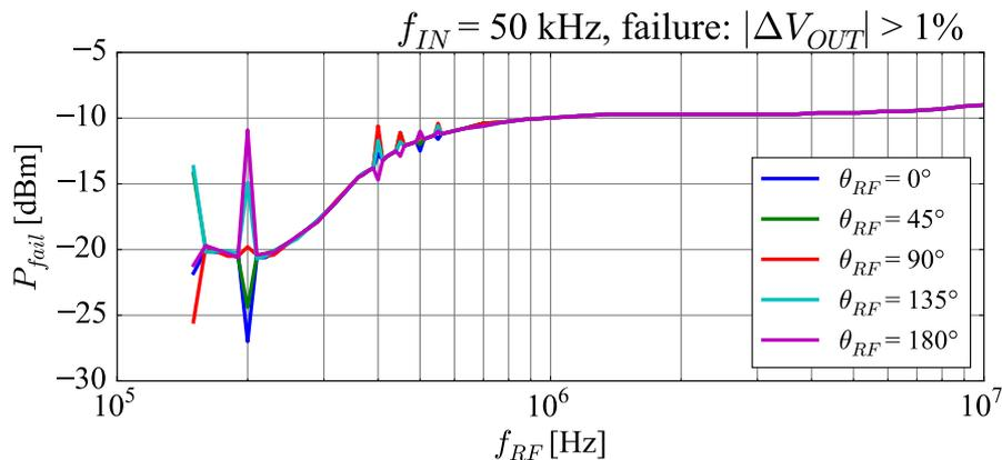
**Figure C.7:** The simulated DPI characteristic of the amplifier in the nonlinear region with  $V_{in,pk} = 50$  mV,  $f_{IN} = 50$  kHz for several values of the initial RF disturbance phase  $\theta_{RF}$  [35].
