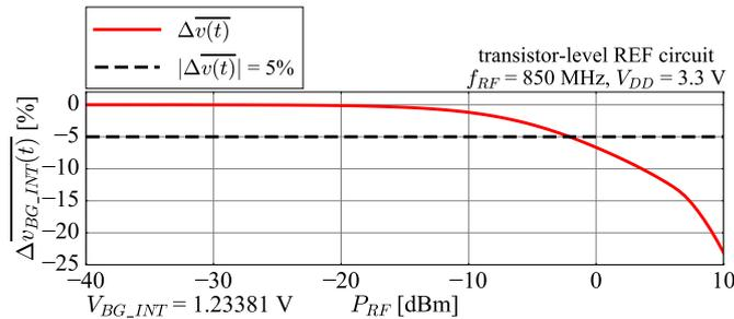
**Figure 3.9:** The RF-induced DC-shift of the BG output signal  $v_{BG\_INT}$  as a function of RF forward power  $P_{RF}$ , expressed as a percentage of the DC operating point value  $V_{BG\_INT} = 1.23381$  V. The limit line of 5% represents a DC-shift of 61.7 mV, and it is crossed at -2 dBm [38].
