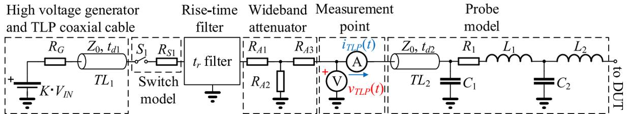
**Figure 4.2:** Mixed lumped-distributed model of the TLP generator [44].
