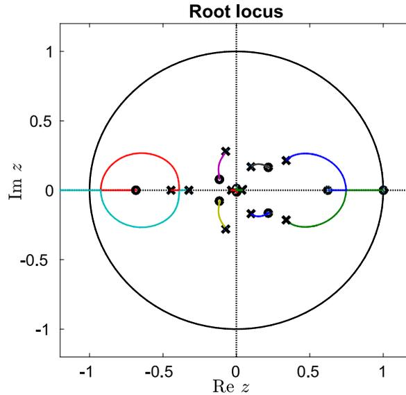
**Figure 3.16:** The root locus of a discrete-time system with 10 poles and 10 zeroes obtained using MATLAB<sup>®</sup>. The open-loop poles are marked by crosses and the open-loop zeroes are marked by circles [42].
