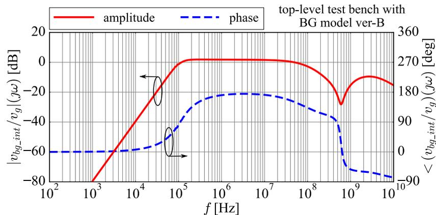
**Figure 3.21:** Frequency response associated with the closed-form solution of the voltage perturbation  $v_{bg\_int}$  versus the RF generator  $v_g$  in the top-level test bench with the BG behavioural model instance ver-B.
