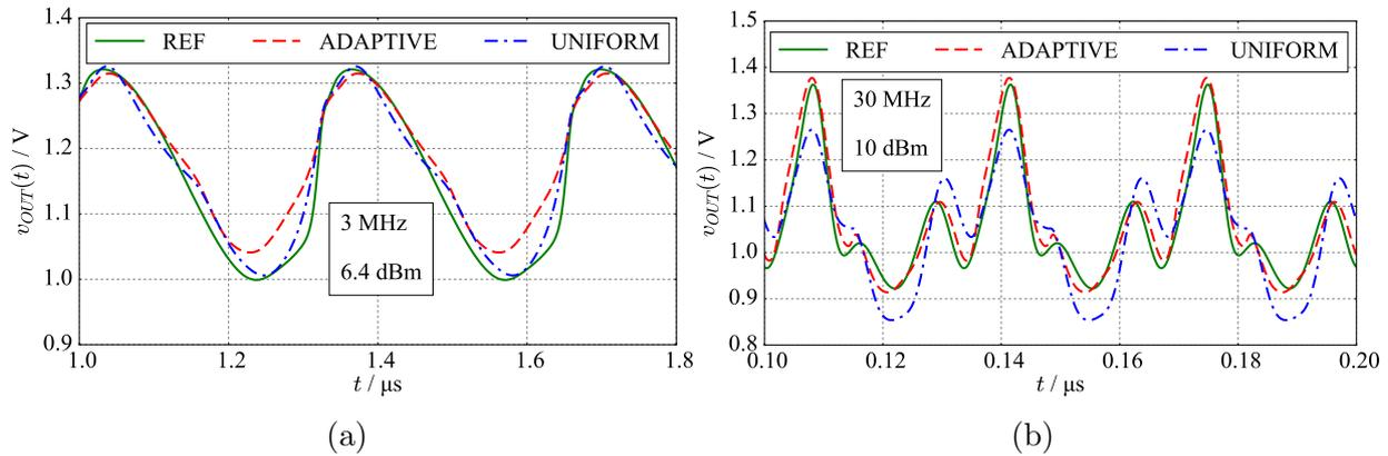
**Figure 2.11:** Comparison of model and netlist of the  $v_{OUT}$  model in: (a) the worst-case MSE point, with  $\text{MSE}_{\text{adaptive}} = 1.60 \cdot 10^{-3}$ ,  $\text{MSE}_{\text{uniform}} = 5.09 \cdot 10^{-4}$ , (b) the highest THD point, with  $\text{MSE}_{\text{adaptive}} = 1.00 \cdot 10^{-3}$ ,  $\text{MSE}_{\text{uniform}} = 4.59 \cdot 10^{-3}$  [37].
