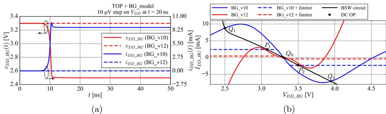
**Figure 3.13:** (a) Time-domain behaviour of the BG model instances v10 and v12 in the top-level test bench under a 10  $\mu$ V step on the REF supply pin at  $t = 20$  ns, (b) DC characteristics of the transistor-level BSW circuit, and the BG behavioural model instances v10 and v12 with and without an ESN input voltage limiter [41].
