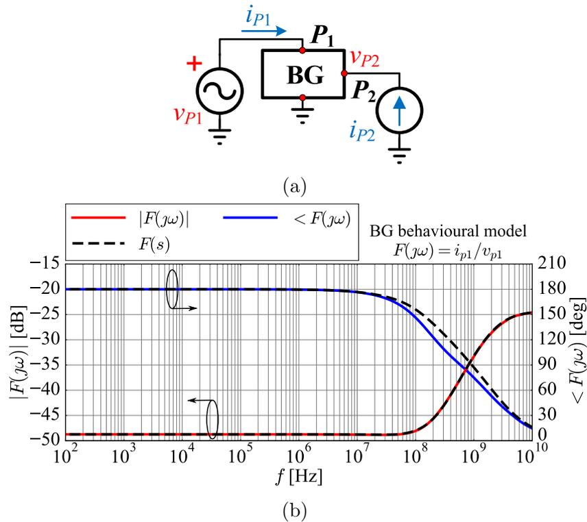
**Figure 3.17:** (a) AC test bench for simulating the small-signal behaviour of the BG behavioural model, (b) frequency response  $F(j\omega)$  of the ESN that models the admittance seen looking into the port  $P_1$  of the BG behavioural model (solid lines), and the frequency response of the fitted transfer function  $F(s)$  with 3 poles and 3 zeroes (dashed lines).
