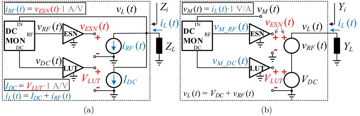
**Figure 3.5:** The extended nonlinear impedance model architecture that enables modelling the DC and RF behaviour of the modelled circuit independently, using separate DC and RF sub-models: (a) based on voltage-controlled current sources, (b) based on current-controlled voltage sources [38].
