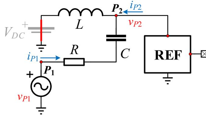
**Figure B.12:** AC test bench for calculating the small-signal behaviour of the bias-tee network with a  $50 \Omega$  RF generator.  $V_{DC} = 3.3 \text{ V}$ ,  $R = 50 \Omega$ ,  $L = 430 \mu\text{H}$ ,  $C = 6.8 \text{ nF}$ .
