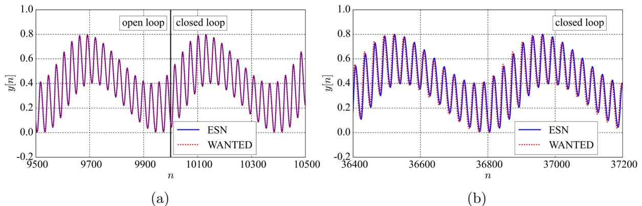
**Figure 2.16:** The behaviour of the ESN model of the oscillator with a feedback connection: (a) in the “teacher forcing” phase during the first  $10 \cdot 10^3$  samples, (b) during the autonomous phase.
