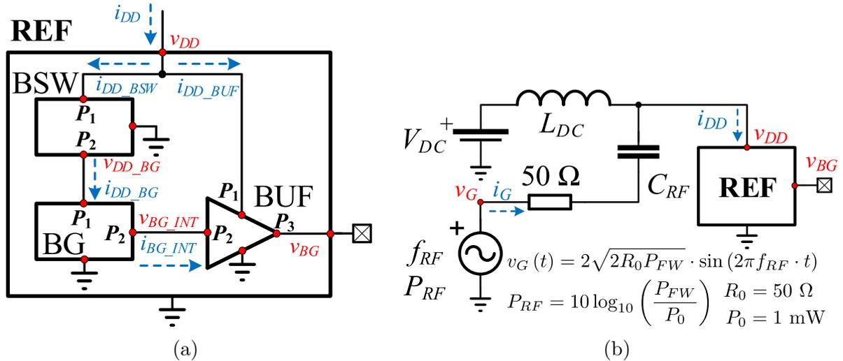
**Figure 3.6:** (a) The buffered voltage reference circuit (REF), consisting of three subcircuits: bulk switch BSW, bandgap BG, and output buffer BUF, (b) the top-level test bench for simulating injection of a single-tone RF interference signal into the supply pin of the REF circuit using a 50- $\Omega$  RF generator and a bias-tee network  $V_{DC} = 3.3 \text{ V}$ ,  $L_{DC} = 430 \mu\text{H}$ ,  $C_{RF} = 6.8 \text{ nF}$  [38].
