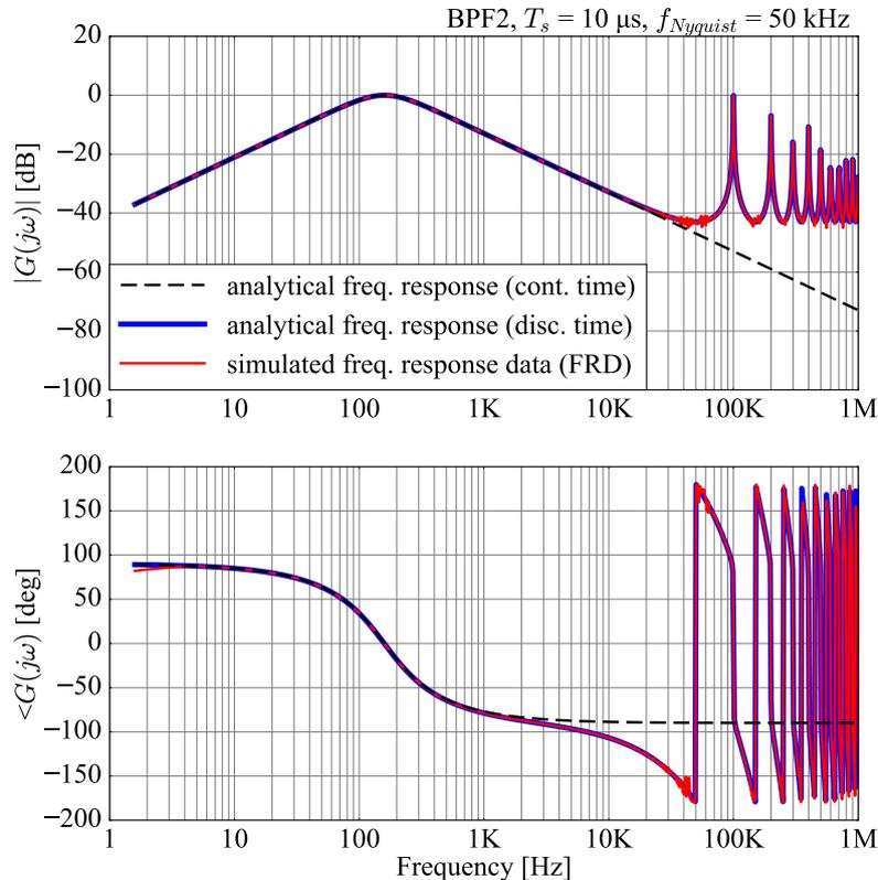
**Figure D.1:** Frequency response data (FRD) of the second-order bandpass filter compared to the analytically calculated frequency response of the discrete-time and continuous-time versions of the filter [42].
