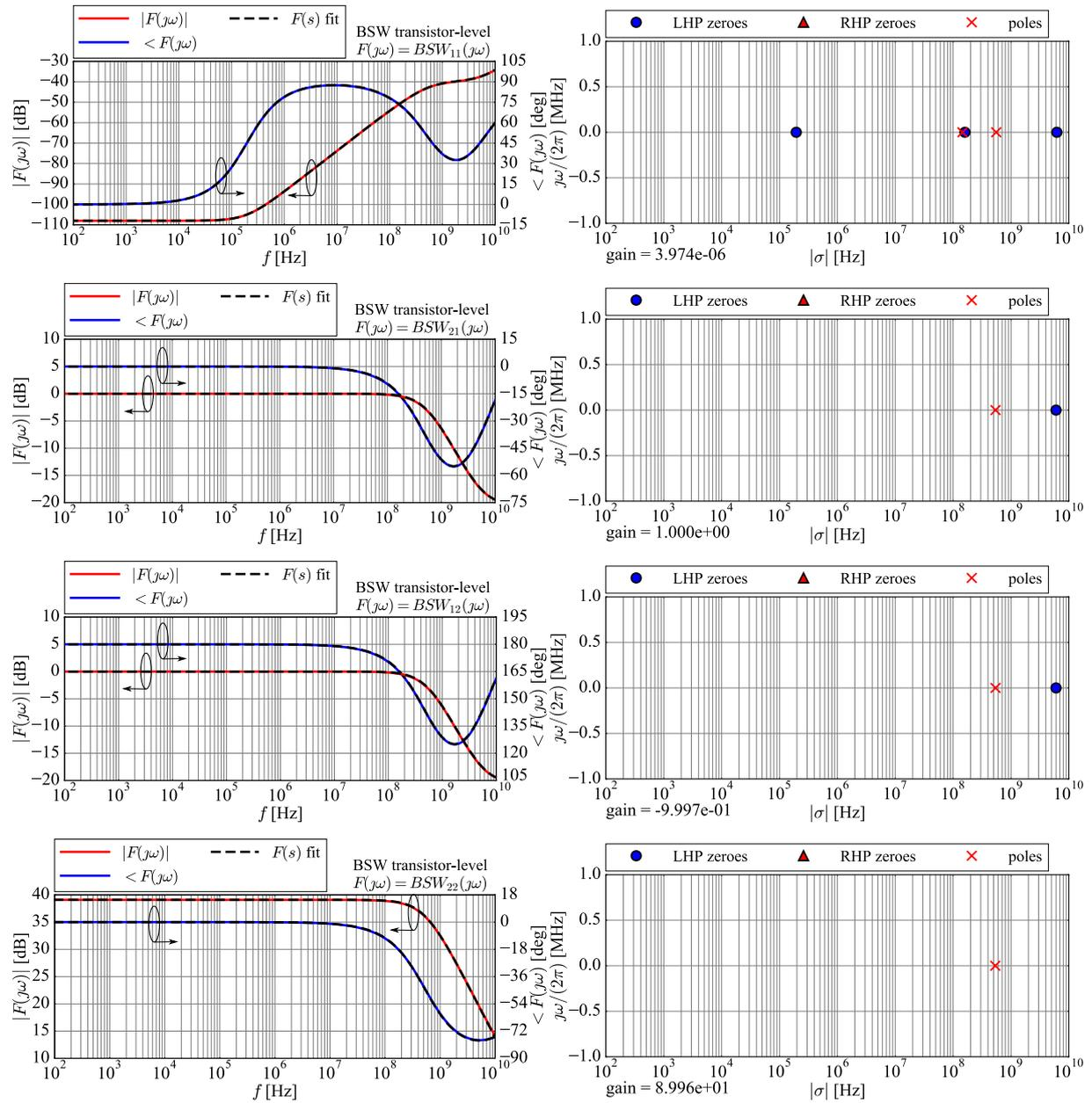
**Figure B.2:** Frequency responses  $BSW_{ij}(j\omega)$  of the transistor-level bulk switch (solid lines), with the associated transfer functions  $BSW_{ij}(s)$  in the  $s$ -domain, where  $s = 2\pi\sigma \pm j\omega$ .
