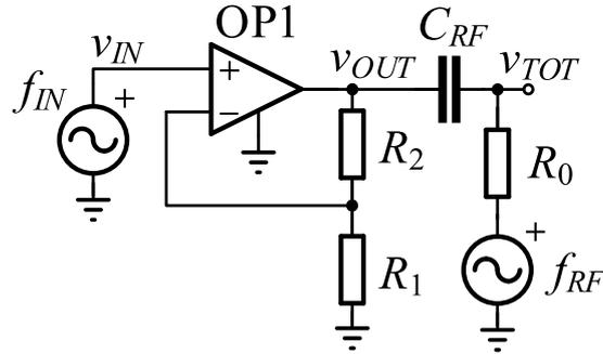
**Figure C.1:** Testbench for DPI simulations of the modelled amplifier with RF disturbance applied to the output pin [35].
