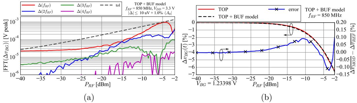
**Figure 3.10:** BUF behavioural model accuracy in the RF forward power sweep of the top-level test bench at 850 MHz, for the BUF output voltage  $v_{BG}$ : (a) amplitude error per harmonic component, with the error bound of  $10 \mu\text{V}$  plus 1% of the fundamental tone amplitude  $|A_0|$ , (b) RF-induced DC-shift error as a percentage of the DC value [38].
