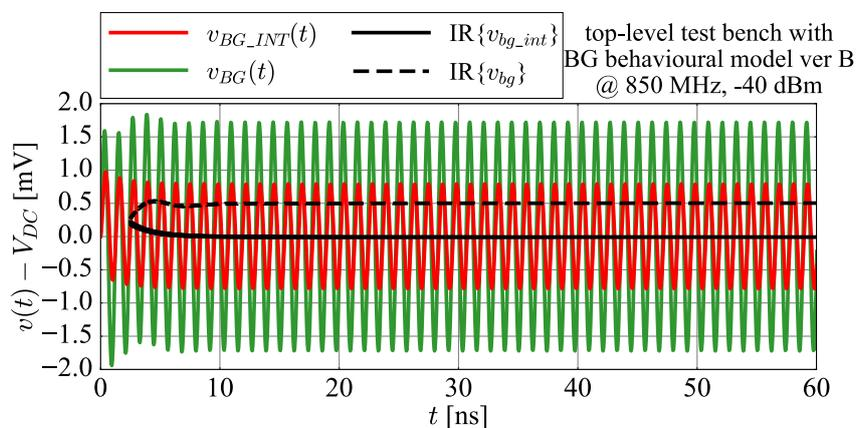
**Figure 3.23:** The initial transients of the voltages  $v_{BG\_INT}(t)$  and  $v_{BG}(t)$  in the TRAN simulation of the top-level test bench with the BG behavioural model instance ver-B at  $P_{RF} = -40$  dBm compared to the impulse responses (IR) of the voltage perturbations  $v_{bg\_int}$  and  $v_{bg}$ .
