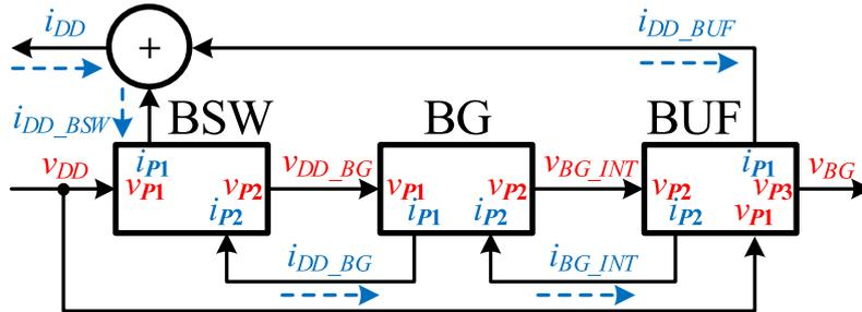
**Figure 3.7:** The flow-diagram of the REF circuit in the top-level test bench, showing the pin voltages and currents for each modelled circuit that are split into the monitored ESN input signals and the driven ESN output signals, as indicated by the direction of the solid arrows [38].
