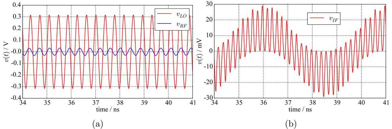
**Figure 2.17:** The input and output test signals obtained using the transistor-level models of the RF mixer “HCBT2” in [49] with  $f_{RF} = 2.4$  GHz,  $f_{LO} = 2.6$  GHz,  $f_{IF,LOW} = 200$  MHz,  $f_{IF,HIGH} = 5.0$  GHz: (a) ESN input signals, (b) ESN output signals. The sampling time is 0.5 ps [34].
