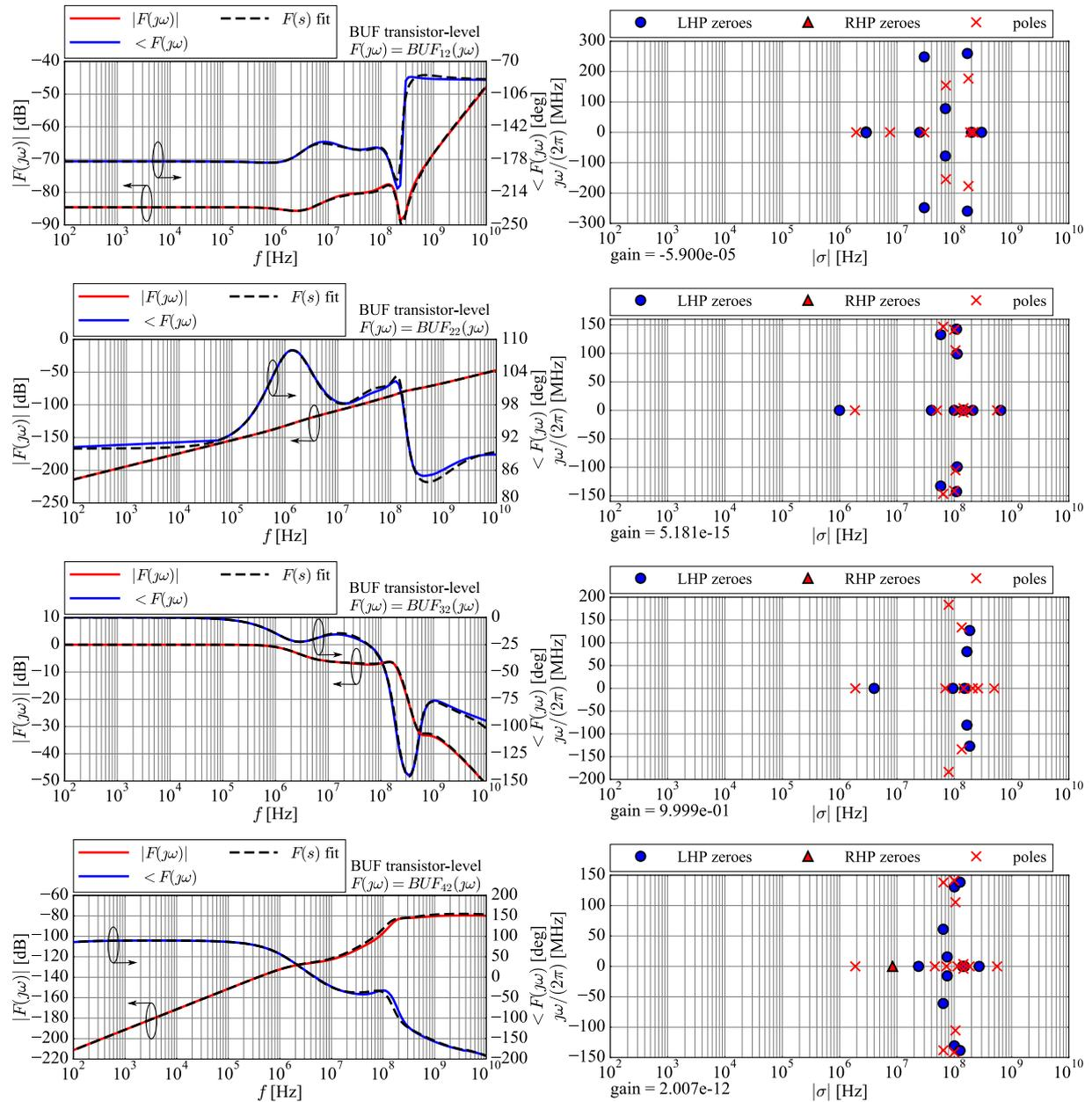
**Figure B.9:** Frequency responses  $BUF_{i2}(j\omega)$  of the transistor-level output buffer in the voltage follower configuration (solid lines), with the associated transfer functions  $BUF_{i2}(s)$  in the  $s$ -domain against the input voltage  $v_{P2}$ , where  $s = 2\pi\sigma \pm j\omega$ .
