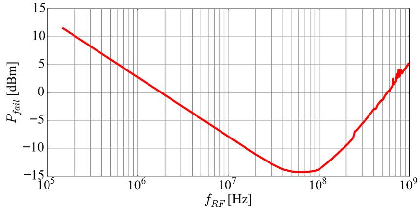
**Figure 3.24:** The DPI characteristic of the transistor-level REF circuit obtained by PSS simulations. The circuit fails if the RF-induced DC-shift of the output voltage  $v_{BG}$  exceeds  $\pm 10\%$  of its nominal value of 1.234 V. The RF frequency step is 10 MHz, and the RF forward power resolution is 0.1 dB [36].
