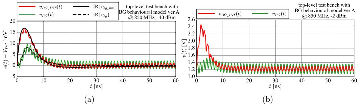
**Figure 3.22:** (a) The initial transients of the voltages  $v_{BG\_INT}(t)$  and  $v_{BG}(t)$  in the TRAN simulation of the top-level test bench with the BG behavioural model instance ver-A at  $P_{RF} = -40$  dBm compared to the impulse responses (IR) of the voltage perturbations  $v_{bg\_int}$  and  $v_{bg}$ , (b) the initial large-signal transients at  $P_{RF} = -2$  dBm [38].
