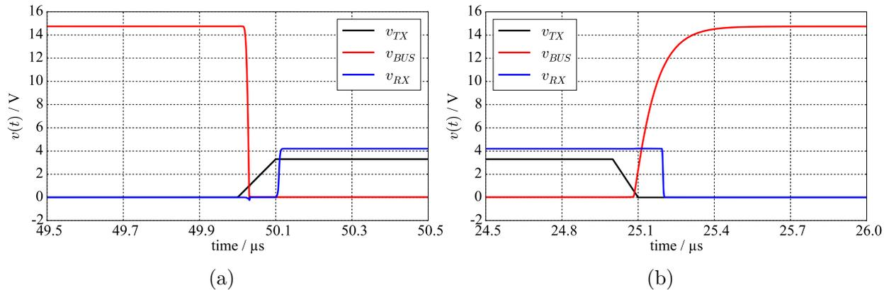
**Figure 2.14:** The input (red) and output (blue) signals obtained using the transistor-level model of the LIN interface with the included parasitic elements: (a) rising edge of the signals, (b) falling edge of the signals. The uniform sampling time is 100 ps [34].
