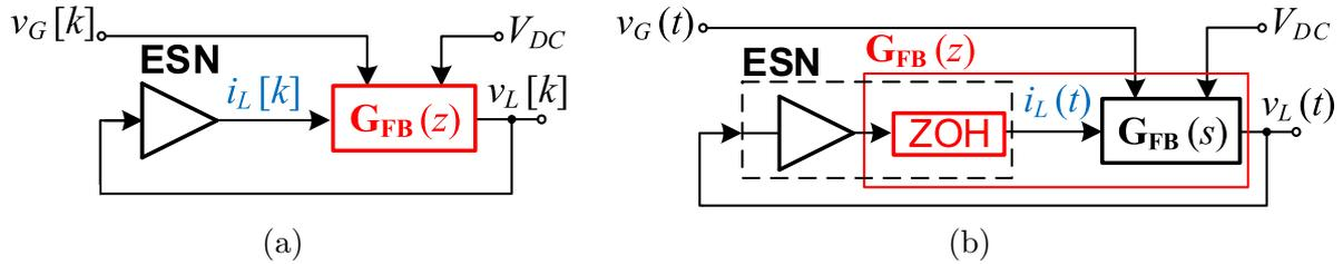
**Figure 3.15:** The flow-diagrams of the feedback loop in the nonlinear impedance model architecture based on the voltage-controlled current source: (a) in the discrete time-domain, (b) in the continuous time-domain [42].
