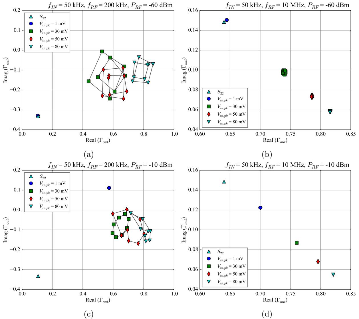
**Figure C.6:** Output reflection coefficient  $\Gamma_{out}$  as a function of the input functional signal amplitude  $V_{in,pk}$  and RF disturbance initial phase  $\theta_{RF}$  swept in steps of  $45^\circ$  at  $f_{RF} = 200$  kHz and  $f_{RF} = 10$  MHz [35].
