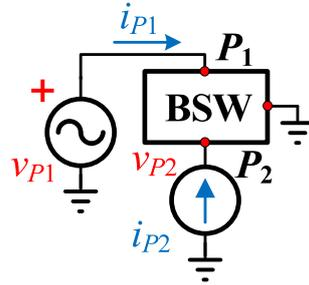
**Figure B.1:** AC test bench for simulating the small-signal behaviour of the bulk-switch.
