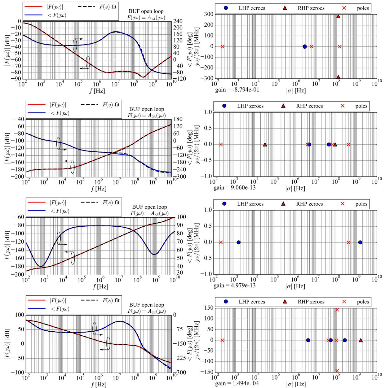
**Figure B.6:** Frequency responses  $A_{i3}(j\omega)$  of the transistor-level output buffer in the open loop (solid lines), with the associated transfer functions  $A_{i3}(s)$  in the  $s$ -domain against the differential-mode input voltage  $v_{2D}$ , where  $s = 2\pi\sigma \pm j\omega$ .
