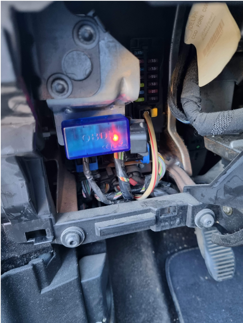
Figure 6.3: ELM 327 device connected to the OBD-II port location in Fiat Grande Punto 2007
