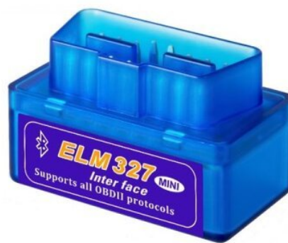
Figure 3.3: ELM-327 OBD-II-to-Bluetooth device [102]
