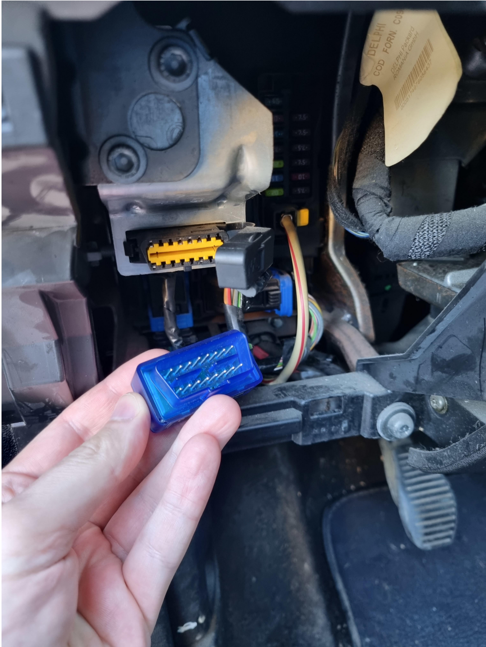
Figure 6.2: ELM 327 device next to the OBD-II port location in Fiat Grande Punto 2007
