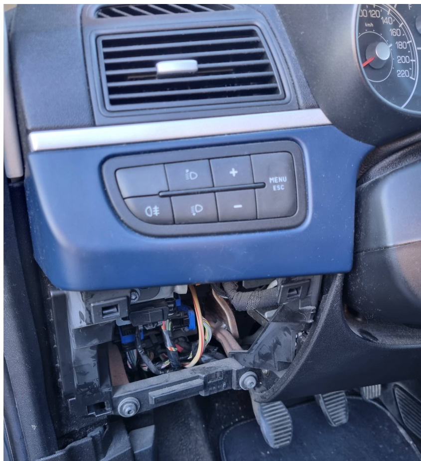
Figure 6.1: OBD-II port location in Fiat Grande Punto 2007
