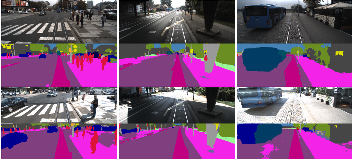
Figure 5.8: Qualitative comparison of model performance during sunny and overcast weather. Model outputs are visualized for presented input images. Each column compares segmentations in different weather conditions. The first column shows how segmentation accuracy degrades in overexposed areas such as the right hand sidewalk, but does not degrade in the middle column example. The rightmost column suggests how flaring in the windshield affects proper segmentation in pixels of the bus.
