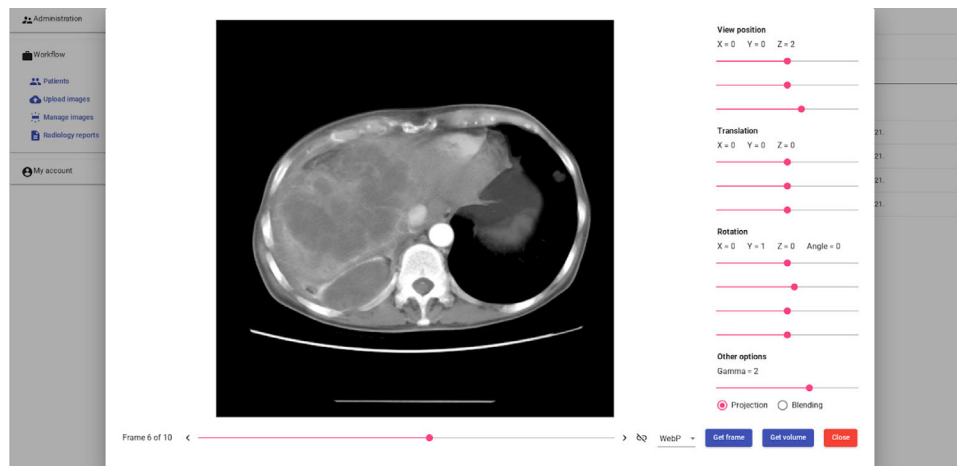
Fig. 4. An example of a remotely rendered slice of a DICOM image. The slider on the bottom is used to select the frame. The menu on the right is used to select the image format.
