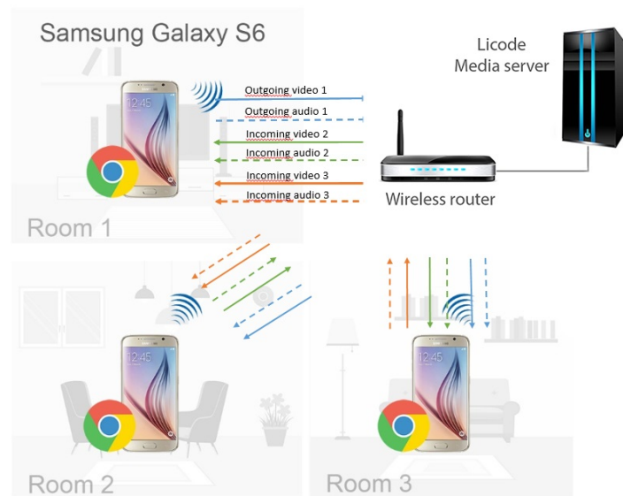
Figure 5.7: System set-up over LAN with Licode media server and Samsung Galaxy S6 (user study US2).
