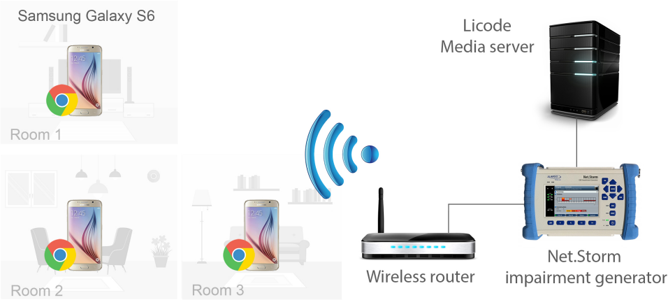
Figure 6.1: Testbed set-up over a LAN (user study US3).
