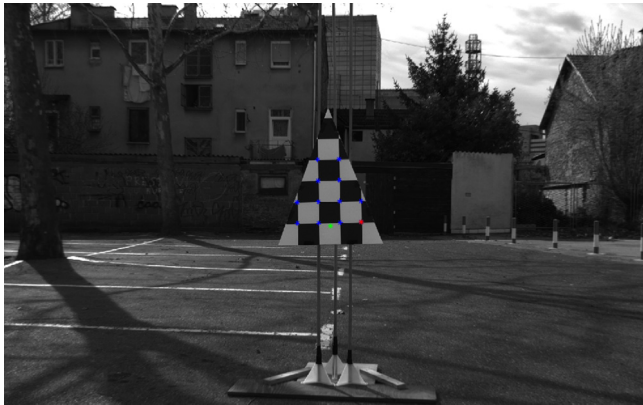
Fig. 2. Front view of the calibration target at the experiment site with detected corners (blue and origin red) and estimated position of the retroreflector origin (green).
