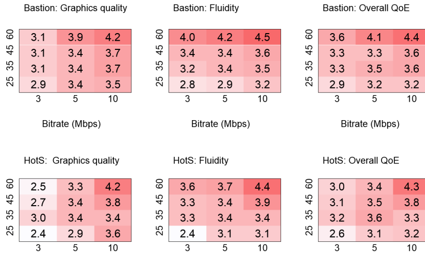
Figure 5.41: Aggregated subjective ratings for each game in Study S6 under different video configurations
