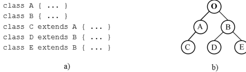
Figure 4.1: a) Class declaration b) Class hierarchy represented by a tree
