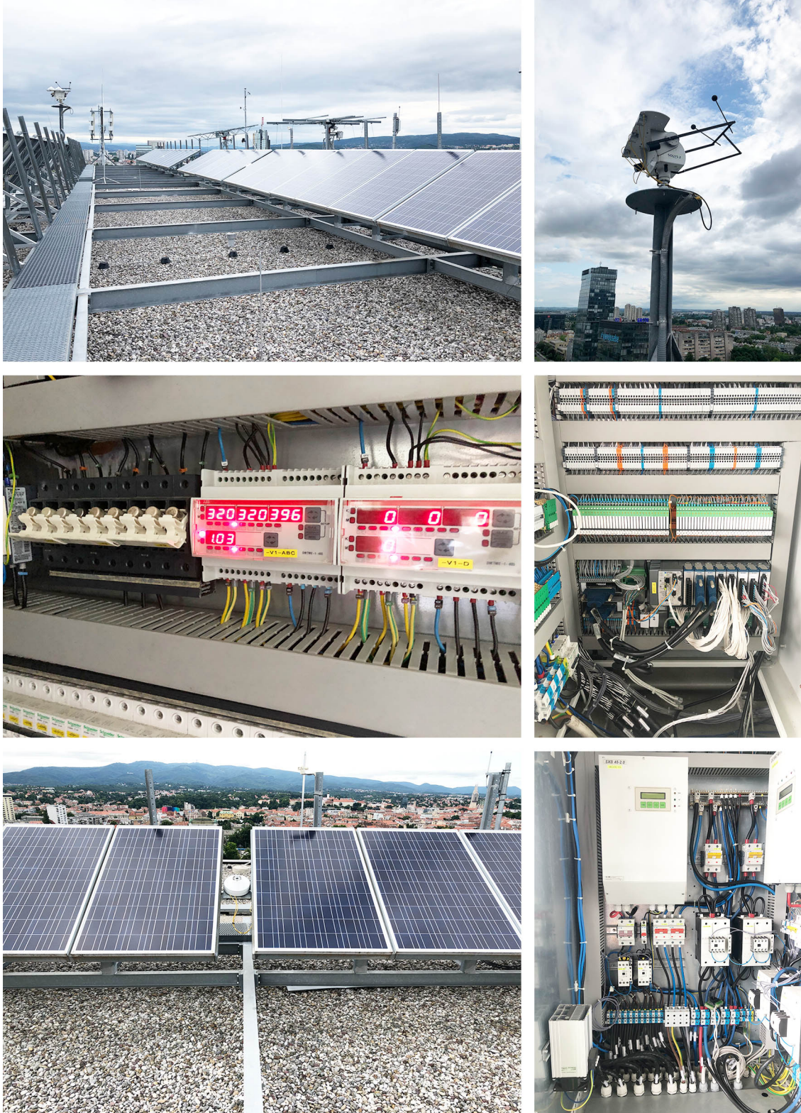
Figure 2.2: Equipment in LARES. From left to right, top to bottom: (i) PV arrays placed at fixed tilt angle to horizontal surface, (ii) Solys2 sun tracker with CHP1 pyrheliometer, two CMP11 pyranometers, and shading balls for diffuse solar irradiance, (iii) three-phase multimeters placed at solar inverter output, (iv) electrical cabinet with microgrid industrial controller and its peripheral, (v) pyranometer to measure solar irradiance incident with the PV array active surface, and (vi) electrical cabinet with microgrid power converters, contactors, automatic circuit breakers etc.
