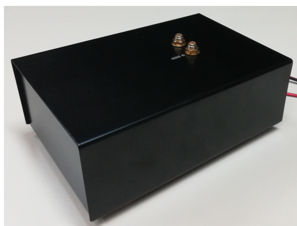
Figure 8.32: NCP in a metal enclosure
