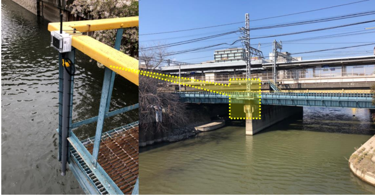
Figure 5.27. Ultrasonic sensor attached to a sensor module used for river water level monitoring.
