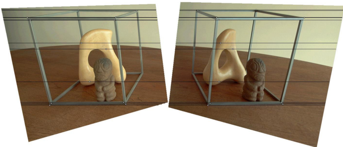
(b) Rectified stereo image pair
