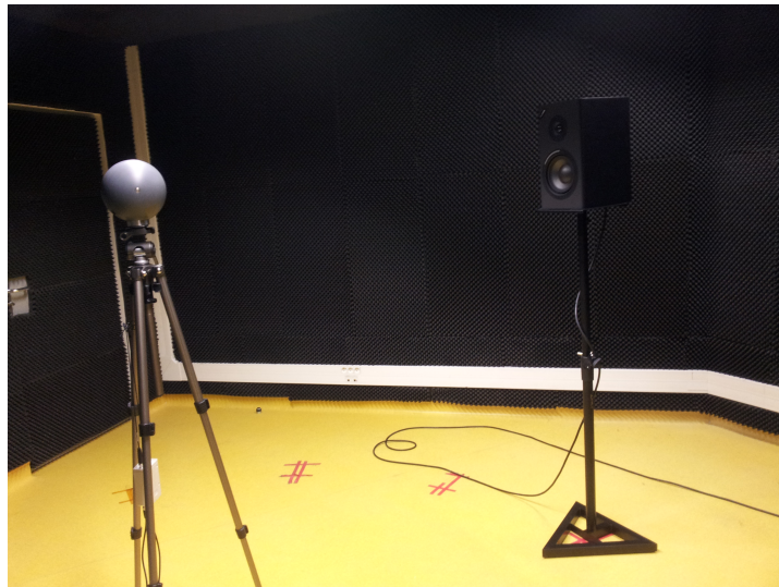
Figure 3.17: Experimental setup: plastic sphere and speaker tripods in the acoustic room. Infrared cameras were measuring the ground-true positions.
