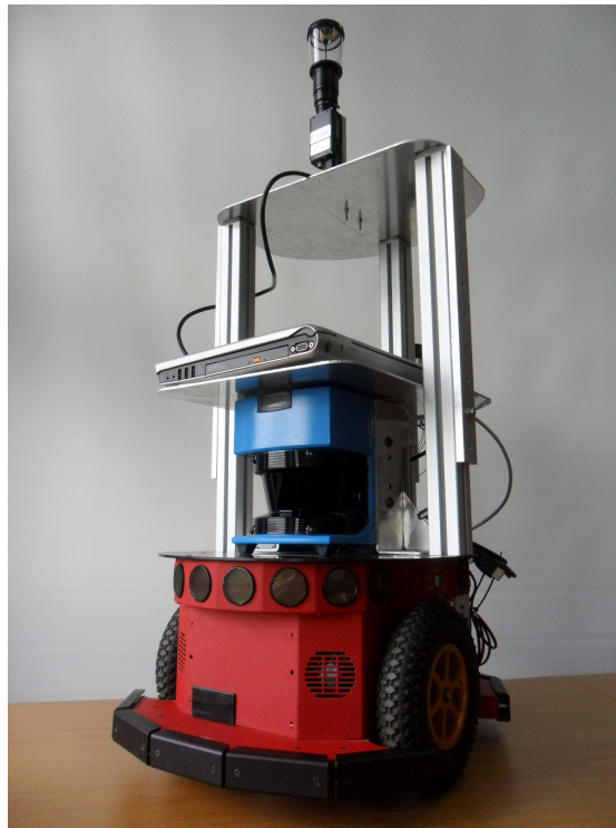
Figure 2.3: Mobile robot equipped with an omnidirectional camera (perspective camera and a hyperbolic mirror)
