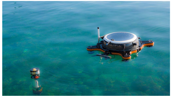
Fig. 2: Autonomous Surface Vehicle H2Omni-X and Sensor Unit
