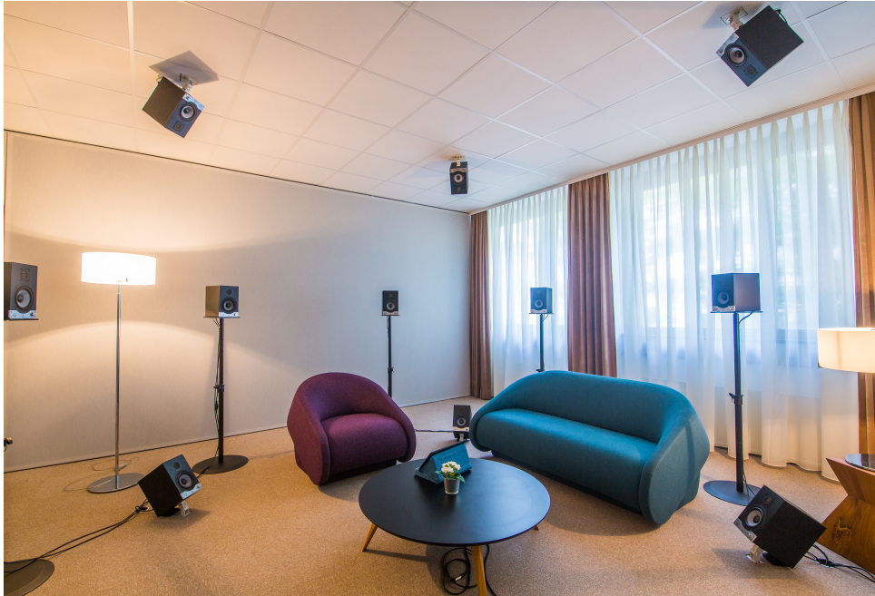
Slika 2.15: Ambisonics postava u TGM ( The school of technology ) u Beču, Austrija [77].
