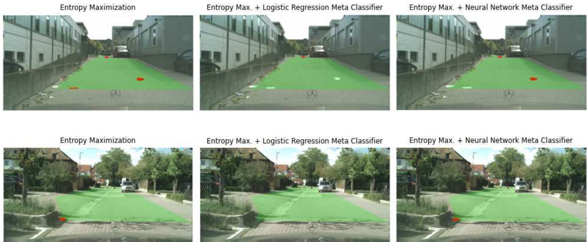
Figure 5.5: Examples of logistic regression outperforming neural network meta classifier. In the first row, logistic regression meta classifier successfully removes OoD object predictions not marked as OoD according to the ground truth segmentation mask (papers on the left and a plastic bag on the right) while neural network meta classifier does not remove the plastic bag. We find this interesting because in this example, neural network meta classifier shows a better generalization ability. In the second row, segmentation network marks part of the road as OoD. It is successfully removed by logistic regression while the neural network meta classifier does not remove it.
