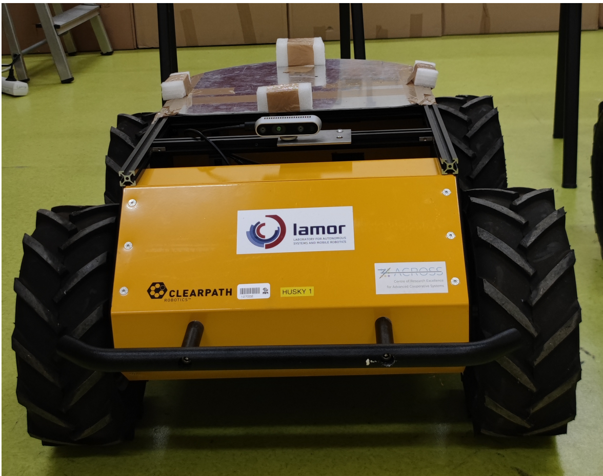
Figure 3.2: Clearpath Husky robot
