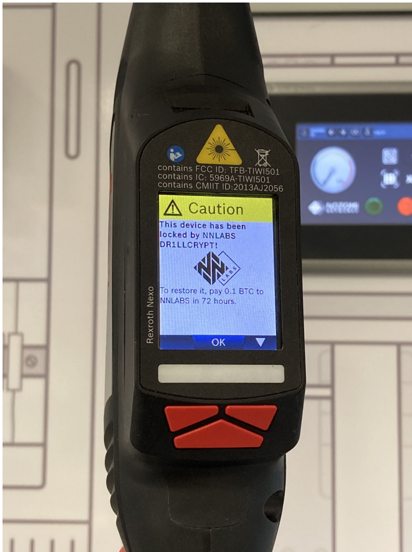
Figure 3.1: A network-connected Bosch Rexroth torque wrench, infected with ransomware while testing vulnerabilities
