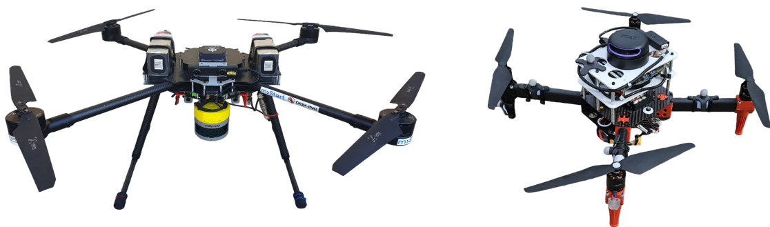
Figure 3.7: Quadcopters used in experiments - Kopterworx UAV with equipped Velodyne VLP-16 LiDAR sensor and ZED stereo camera (left), and modified Hexsoon EDU-450 with SLAMTEC RPLIDAR-A3 2D LiDAR used for obstacle detection (right).
