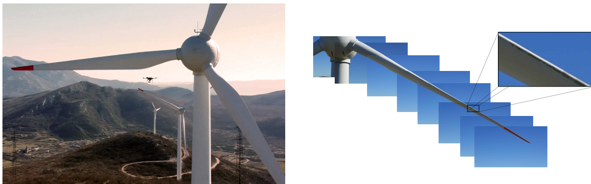
Figure 2.2: Autonomous wind turbine inspection conducted by an UAV (left). High-resolution images acquired during the survey mission that are used for damage assessment on the wind turbine blades (right).
