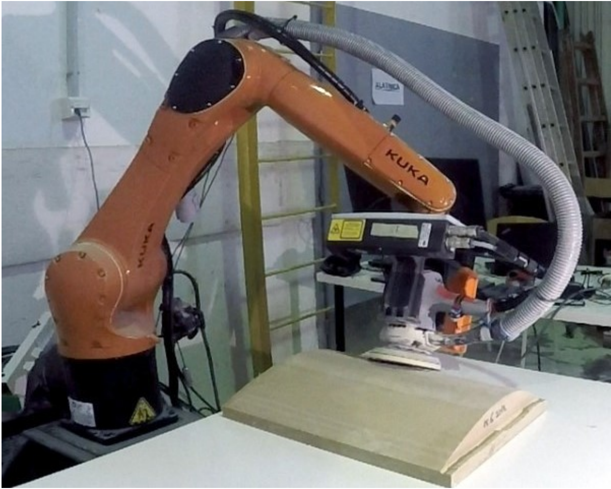
Figure 6.1: Showing compliance control setup involving industrial manipulator KUKA KR10 performing delicate sanding of complex surfaces in an industrial scenario.
