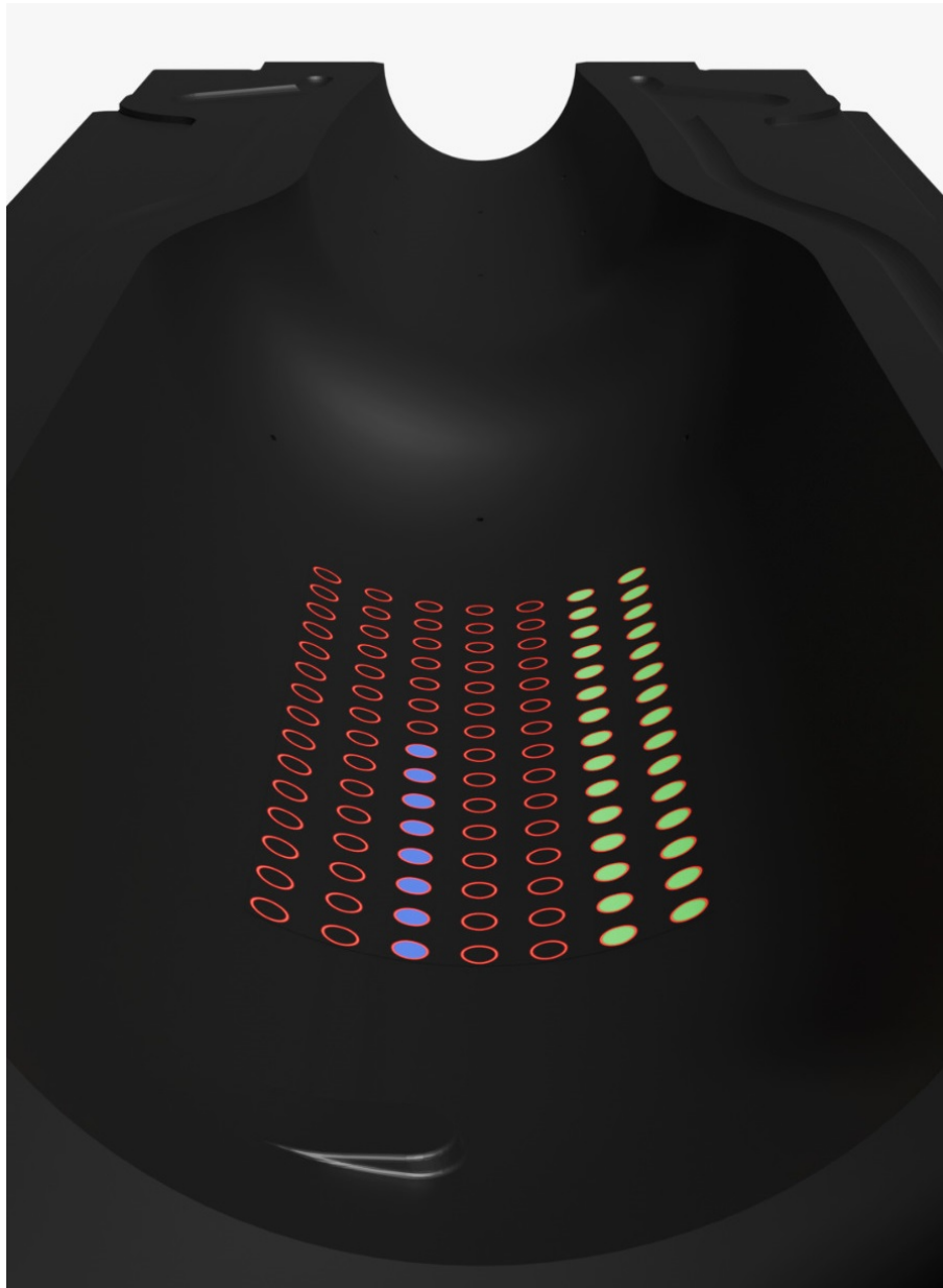
Figure 6.14: Illustrating robotic system performance: Red circled points are pilot holes (1mm deep) optimized for experiment consistency and post-analysis hole localization. Blue filled dots indicate operator-drilled holes, and green filled dots represent holes completed by the robot.
