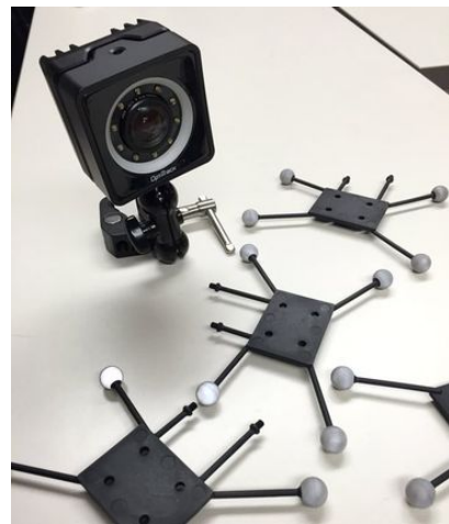
(c) Optitrack markers and camera 7
