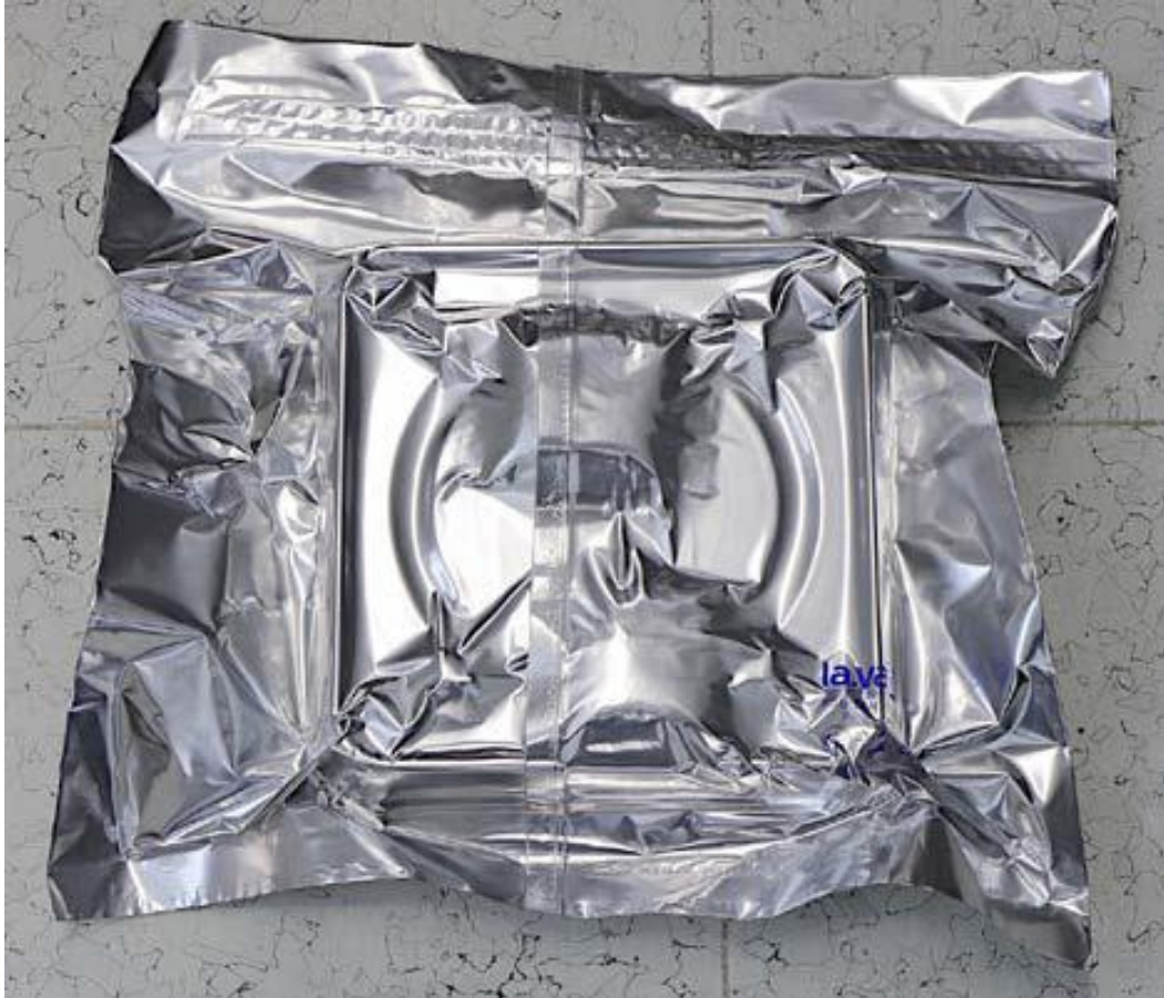
Figure 4.7. Wafer box was placed in an ESD vacuum sealer bag and evacuated so that it can be safely stored in a cooler at T = -22\text{ }^{\circ}\text{C} .
