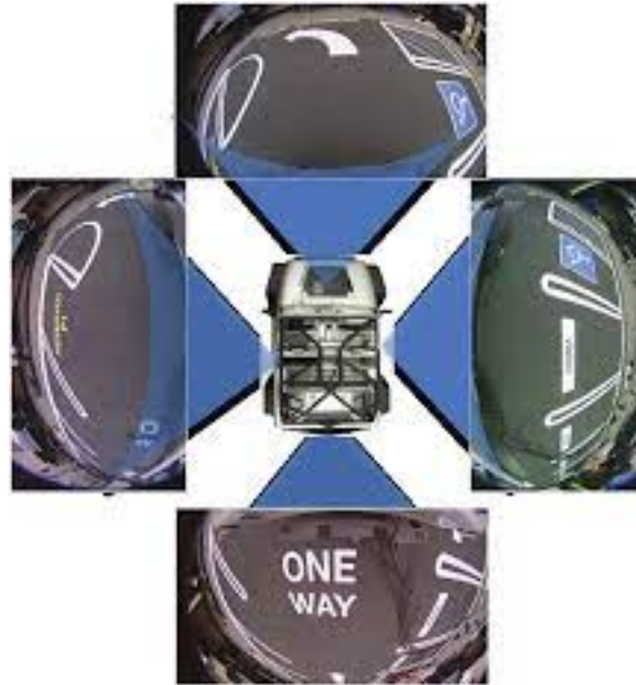
Figure 1.1: An example of a vehicle surround-view capture system with four fish-eye lens cameras on the four sides of the vehicle, [2]. The four images around the center show the camera view from the four fish-eye lens cameras placed on the vehicle.
