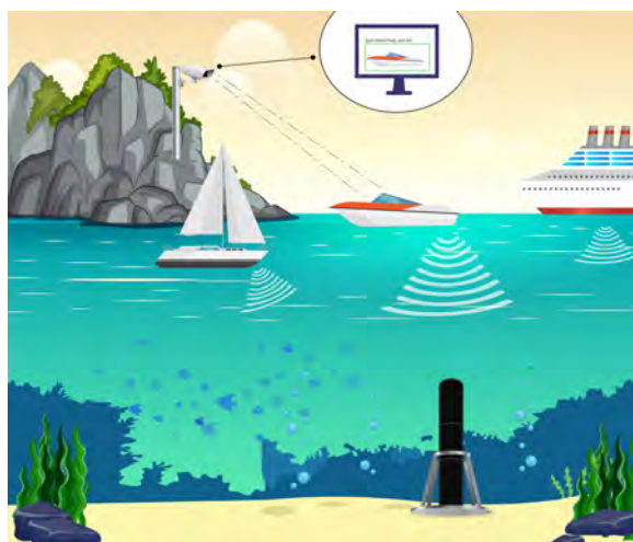
(a) Illustration of the acoustic-optic testbed for quantifying the URN of VOO by using synchronized optical measurements from a shore-based camera and an acoustic recorder positioned at the seabed.
