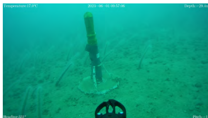
(b) Picture of the underwater acoustic recorder at the deployment site.
