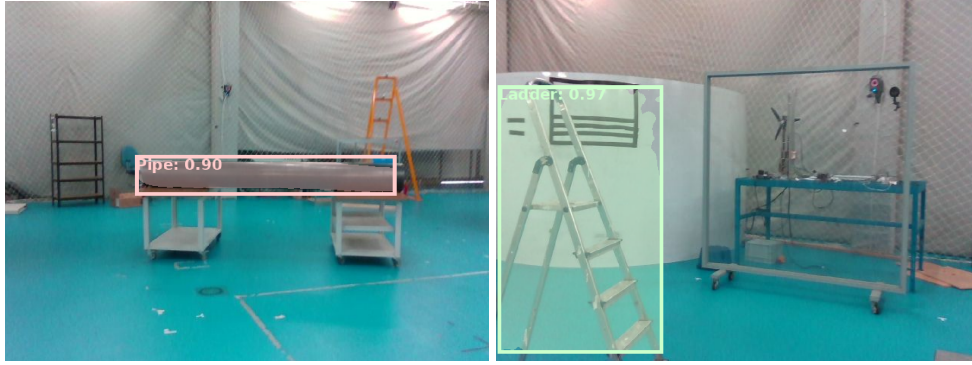
Figure 4.13: Results of the mmdetection algorithm using RetinaNet. The model, trained specifically for construction site environments, effectively detects pipes and ladders. The detection is performed in the real-world scenario.
