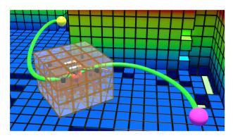
FIGURE 3. A UAV executes a planned path (green) from a start point (pink) to a target point (yellow) in an OctoMap. A rectangular prism-shaped state validity checker (transparent white and orange) simplifies the representation of the UAV. The validity checking is performed for each point (orange point) of the planned path.
