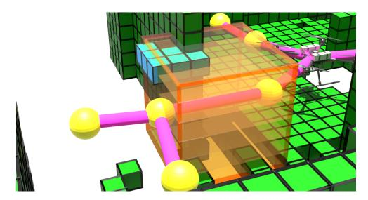
**Figure 4.10:** An illustration of the proposed Recursive Shadowcasting algorithm in the OctoMap. The algorithm is performed inside the cuboid centered at the path edge, on each 2D slice (planes inside the cuboid). The results of the RSC are shown on the first OctoMap slice, where the cyan voxels represent unknown voxels while the grey voxel is not taken into account for the information gain calculation.
