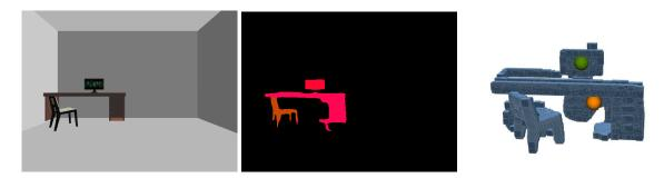
**Figure 4.12:** Semantic segmentation of simple features (table, chair and monitor). The semantic segmentation is performed with an HRNet model trained on the ADE20K dataset. Once the objects are semantically segmented, the 3D position of each object is extracted and colored in a specific color matched to the object.
