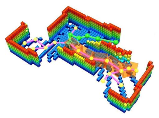
**Figure 4.11:** The UAV body (cyan color) denotes the first point of the path. Orange cuboids along the path of the RRT illustrate the volume where the information gain is computed. A green path with green waypoints is the best path. Pink paths with yellow waypoints are other paths of the RRT.
