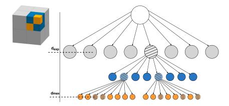
**Figure 4.5:** The structure of an octree and the cube-shaped space it represents. A representation of frontier voxels at the maximum depth  $d_{max}$  and their corresponding parent nodes at the chosen exploration depth  $d_{exp}$ .
