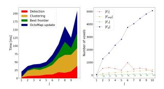
Fig. 8. Large scenario metrics for  $r_{max}=0.5~{\rm m}$ ,  $r_{exp}=2~{\rm m}$ , bandwidth = 2. On the left, the computation times for significant modules in each iteration j are shown. On the right, a graph shows the number of voxels in each iteration.
