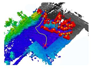
Fig. 1. A snapshot of the proposed method in action. Grey and white parts of the OctoMap represent the unexplored and green/blue explored environment. Red voxels represent the frontier and yellow voxels are centroids of frontier point clusters. A UAV explores the environment by planning a trajectory towards the selected cluster centroid.
