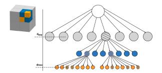
Fig. 4. The structure of an octree and the cube shaped space it represents. An instance of frontier voxels at  $d_{max}$  and their parents on the desired exploration depth  $d_{exp}$ .
