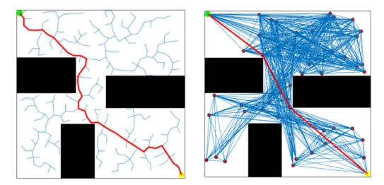
**Figure 4.8:** Graph search algorithms based on sampling. The green, yellow and red points denote the starting, ending and sampled points, respectively, and the red curve represents the global path. On the left, the performance of the RRT is shown, while on the right, the path planned with the PRM is visualized [95].
