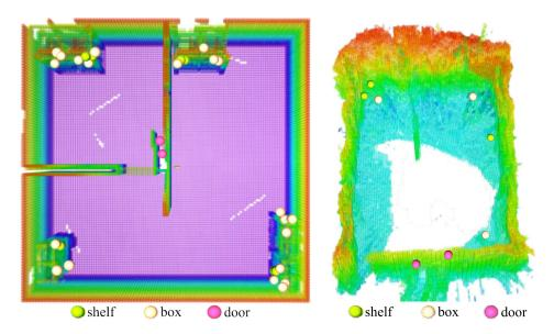
**Figure 4.14:** The OctoMap of the warehouse environment in the simulation and in the real-world experiment is shown on the left and right respectively. The transparency effect is applied on the OctoMap and detected objects during the exploration are shown. Shelves, boxes and doors are shown with different colors on the map.
