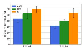
FIGURE 11. Total distance traveled in the simple environment for the ASEP, MRF and CF. Data are given as means of 10 runs with standard deviations.
