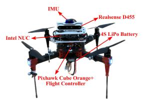
FIGURE 13. A Hexsoon EDU-450 quadcopter equipped with a Intel NUC, a Realsense D455 camera, an IMU, a battery and a flight controller.
