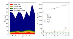
Fig. 13. Outdoor scenario metrics for  $r_{max} = 0.5$  m,  $r_{exp} = 2$ , bandwidth = 2. On the left, the computation times for significant modules in each iteration j are shown. On the right, a graph shows the number of voxels in each iteration.
