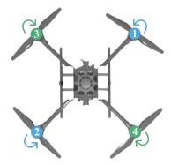
Figure 2.1: The spin direction of the propeller motors on the quadcopter.
