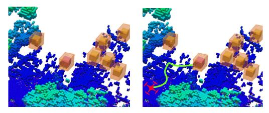
**Figure 4.7:** Information gain calculation for the potential exploration targets is shown on the left. Cubes are placed around the candidates and the information gain is proportional to the number of unknown voxels within the cubes. The UAV selects the best frontier according to Eq. 4.6, plans the path and navigates toward the target.
