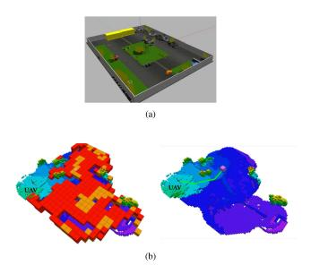
Fig. 10. Large exploration scenario. (a) Gazebo world (b) An instance of the exploration process. Global frontiers are marked red, candidates yellow while the best frontier voxel  $\mathbf{v}_{bf}$  is marked pink. The UAV planned a path (green) to the best frontier voxel (target).
