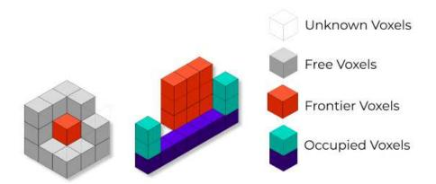
**Figure 4.3:** Illustation of a 3D frontier detection. The voxels are shown in 3D space which is a more complex, volumetric space where the boundary between free (gray) and unknown (transparent) voxels represents frontier (red) voxels.
