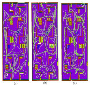
FIGURE 10. The OctoMap of the complex scenario created by the ASEP, MRF and CF, respectively, with planned paths, at the resolution  $r=0.2\ \mathrm{m}$ .
