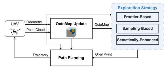
**Figure 4.1:** Overall schematic diagram of the 3D exploration system. The system input module generates odometry data and point cloud data that produce input data for OctoMap creation. The exploration strategy generates a goal point towards which the robot plans its path and navigates.
