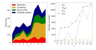
Fig. 6. House scenario metrics for  $r_{max} = 0.25$  m,  $r_{exp} = 1$  m, bandwidth = 2. On the left, the computation times for significant modules in each iteration j are shown. On the right, a graph shows the number of voxels in each iteration.
