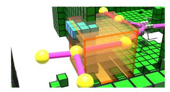
Fig. 1. An illustration of the proposed Recursive Shadowcasting algorithm in the OctoMap. The algorithm is performed inside the cuboid centered at the path edge, on each 2D slice (planes inside the cuboid). The results of the RSC are shown on the first OctoMap slice, where the cyan voxels represents unknown voxels while the grey voxel is not taken into account for the information gain calculation.
