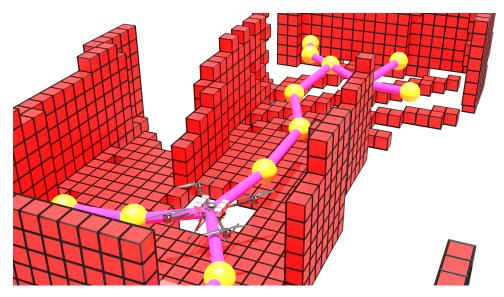
**Figure 4.9:** An illustration of the RRT node and path generation. Pink paths with yellow waypoints (nodes) are the result of the RRT. The origin of the RRT is at the position of the UAV. The OctoMap is shown in red for better visualization.
