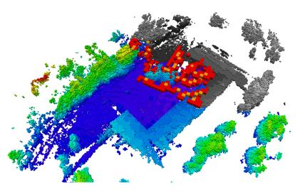
**Figure 4.6:** Results of mean-shift clustering during real-world experiments within this thesis. Grey and white parts of the OctoMap represent the unexplored and green/blue explored environment. Red voxels represent the frontier and yellow voxels are centroids of frontier point clusters, the output of the mean-shift algorithm.
