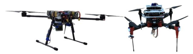
**Figure 1.2:** UAVs used in outdoor and indoor experiments. On the left is a *Kopterworx* quadcopter, a custom built quadcopter equipped with a Velodyne VLP - 16 LiDAR sensor. On the right is a *Hexsoon EDU-450* quadcopter equipped with a Realsense D455 camera.
