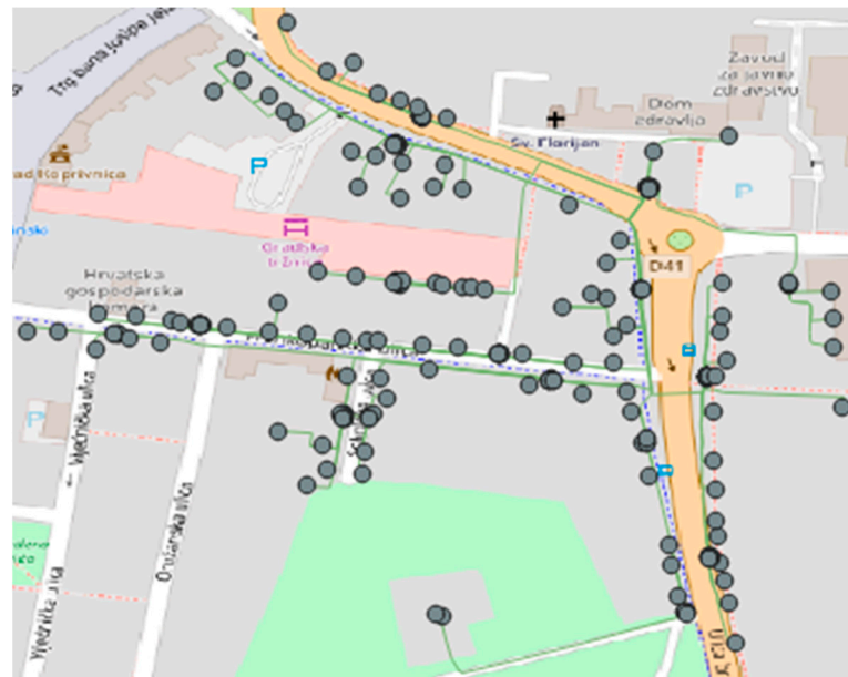
Figure 1. Modelled LV distribution network.
