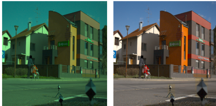
Figure 3.1: Image before and after being chromatically adapted using the von Kries model
