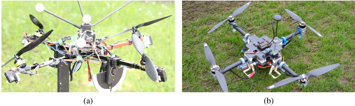
Figure 1.3: The figure shows tilt configuration UAVs. In a) the quadrotor prototype with ability to control the orientation of its 4 propellers is presented [24], in b) a dual-axis tilting propeller is shown [22]. In paper one can find more about design, modeling, simulation and prototyping of such quadrotor.
