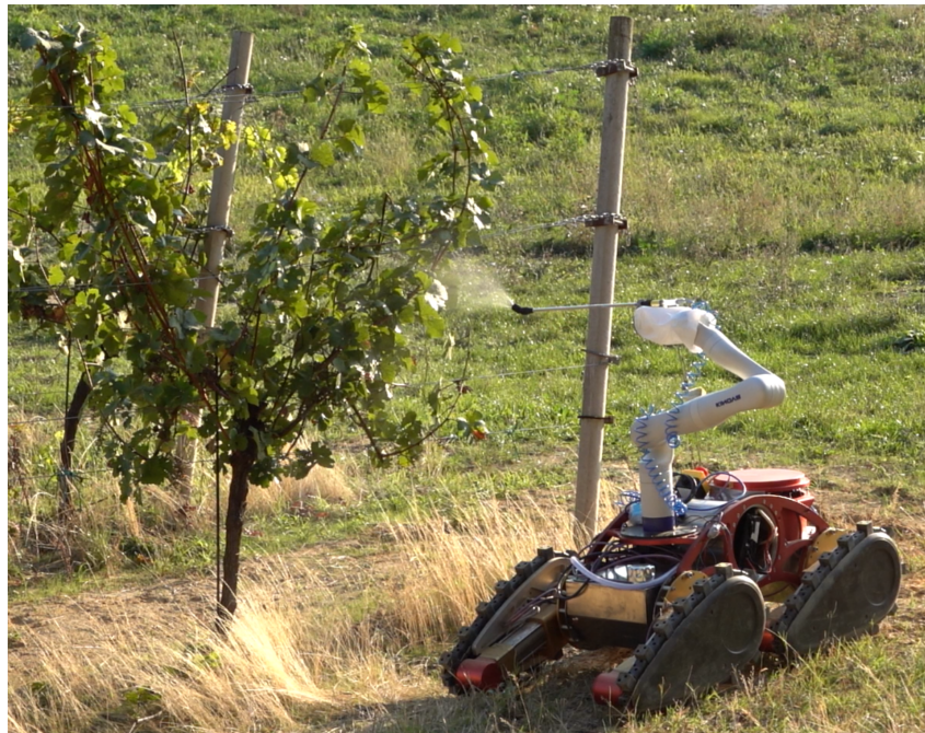
Figure 3.6: Mobile manipulator performing a continuous spraying experiment in a vineyard. A single row of grapevines is sprayed using the presented task space MPC based method. Copyright [8]CC BY 4.0.
