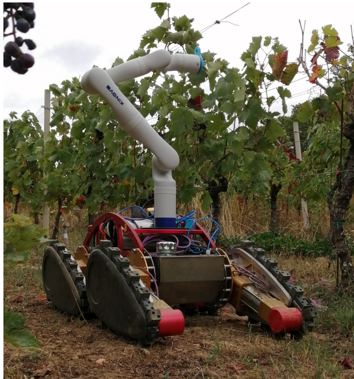
Figure 1.2: A mobile manipulator used in the HEKTOR project and throughout this thesis. It features a custom flipper-tracked vehicle as its mobile base, mounted with a Kinova Gen3 robot arm for the execution of manipulation tasks. Copyright [8]CC BY 4.0.
