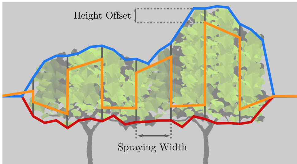
Figure 3.4: Orange line represents the lawnmower trajectory used as the spray frame reference. The upper and lower boundary of the canopy description are represented by a blue and a red line respectively. Copyright [8]CC BY 4.0.
