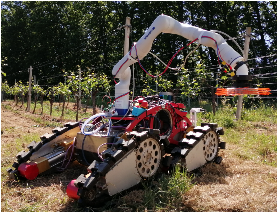
Figure 4.3: Mobile manipulator equipped with a specialized brush-shaped suckering tool in a vineyard. Copyright [58]CC BY 4.0.
