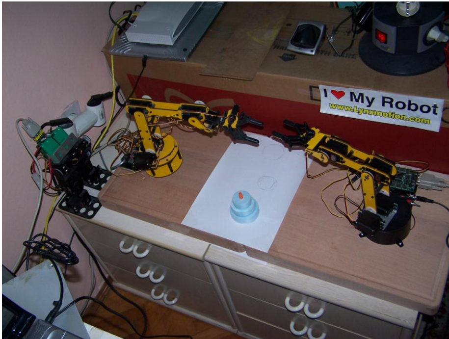
Figure 9.9. The two collaborating robotic arms solving the TOH(3) problem
