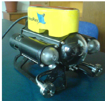
Figure 3.7. VideoRay ROV with vision-based laser distance module.
