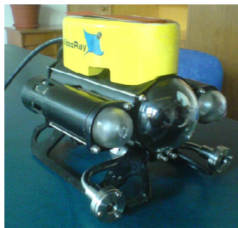
Figure 3.7. VideoRay ROV with vision-based laser distance module.
