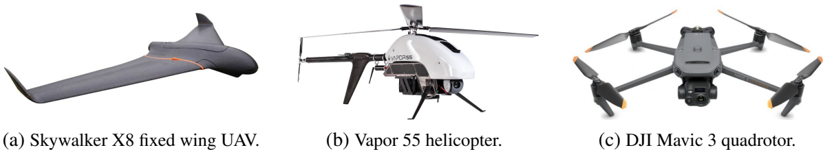
Figure 1.1: Representative examples of three main categories of unmanned aerial vehicles.
