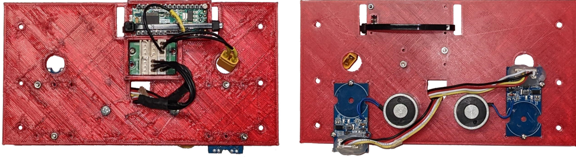
(a) Top plate of the magnetic gripper with the Arduino Nano controller and power distribution board. (b) Bottom plate of the magnetic gripper with Grove Electromagnet controller boards.
