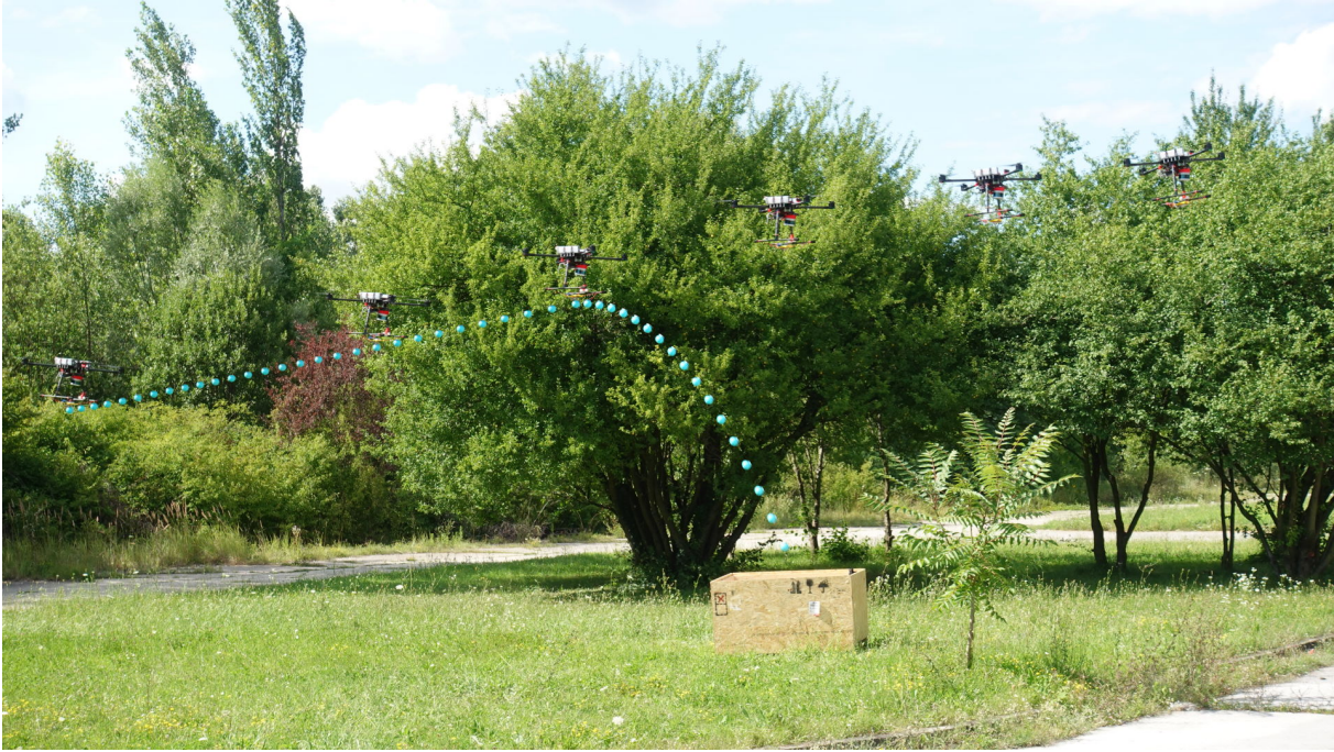
Figure 7.1: An example of the multirotor performing the parabolic airdrop in an outdoor environment. The multirotor steers towards the launch point and releases the payload, after which it executes a stopping motion. After the release instance, the free-fall parabolic trajectory can be observed. Copyright [14] CC BY 4.0 .
