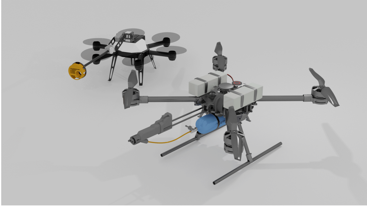
Figure 5.13: The envisioned team consisting of two aerial manipulators for bridge sensor mounting. The right aerial manipulator carries a pressurized tank with the resin component, and applies it on a bridge surface. The left aerial manipulator carries the sensor with the pre-applied hardener component, and glues the sensor on the bridge surface. Copyright [33] CC BY 4.0 .
