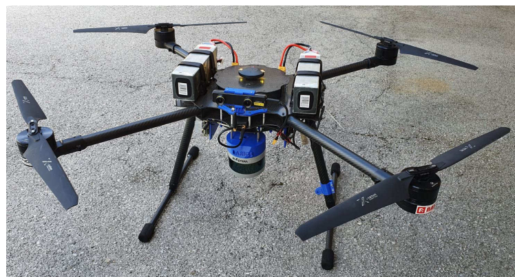
(d) Wind turbine inspection multirotor. Copyright [7] CC BY 4.0.
