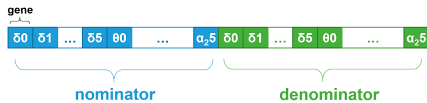
Figure 3. An illustration of a chromosome structure in the proposed optimization problem solution.
