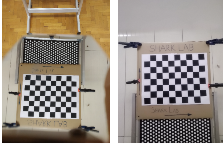
Figure A.8: Example of the original calibration chessboard pair of views (before image flipping and rotation), recorded using back and front camera, respectively. Adapted from [286].
