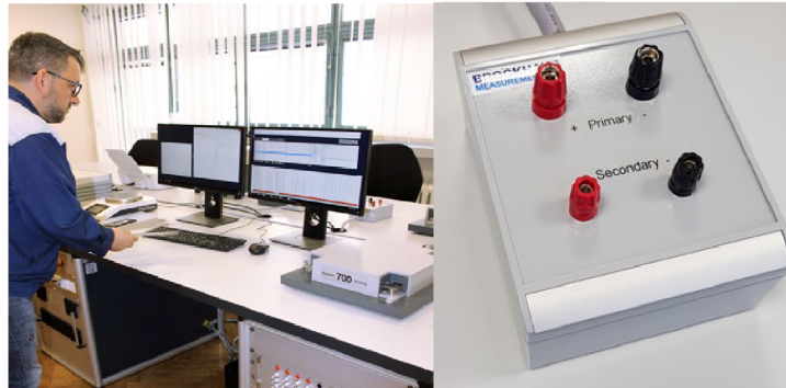
FIGURE 5.4: Laboratory for Testing of Magnetic Materials at the Končar IET Laboratory Center and ring measuring coil sensor used in this research [49].
