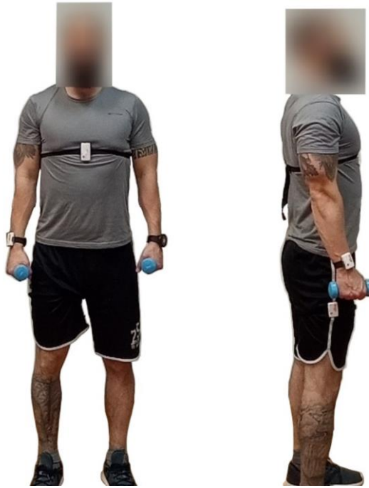
Figure 13 The 3 IMUs positions: 1) right wrist, 2) chest (in middle above the navel)) and 3) right thigh (mid-point, lateral surface)
