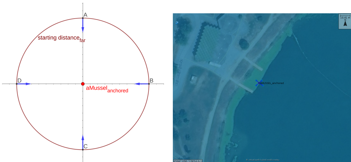
Figure 2.27: Starting positions for docking attempts around an anchored aMussel as envisioned (left) and marked as goalpoints in the Neptus C4I Framework used for aPad mission supervision and control (right) [82].
