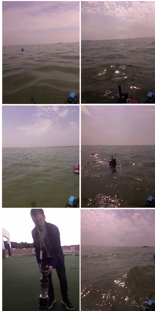
Figure 2.20: Difficult detection examples (output aMussel bounding boxes shown in blue) which neural networks were extremely helpful in resolving - including cases with larger distances, partial visibility, occlusion, wave splashes/partial submersion, bad lighting and weather conditions, and sunlight glare.
