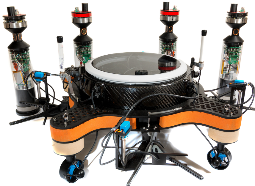
Figure 2.1: The aPad platform and four aMussel underwater sensor nodes.
