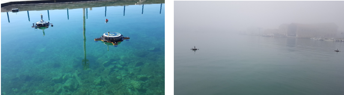
Figure 1.3: subCULTron swarm agents in outdoor testbed pool (left) and in realistic conditions in the Venice Arsenal (right).
