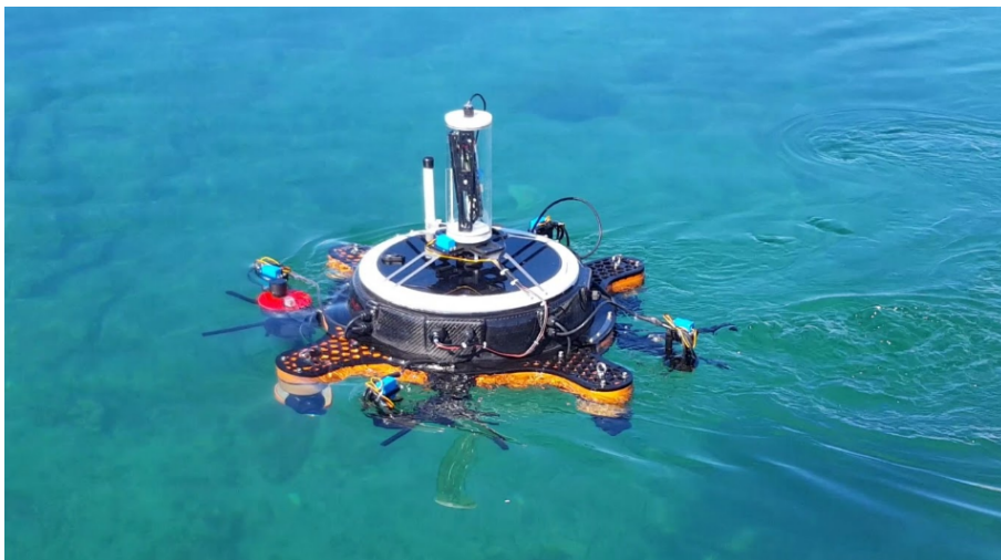
Figure 2.24: aPad with pan mechanism and Kinect sensor docking an aMussel (red cap, left, partially submerged) during outdoor tests.
