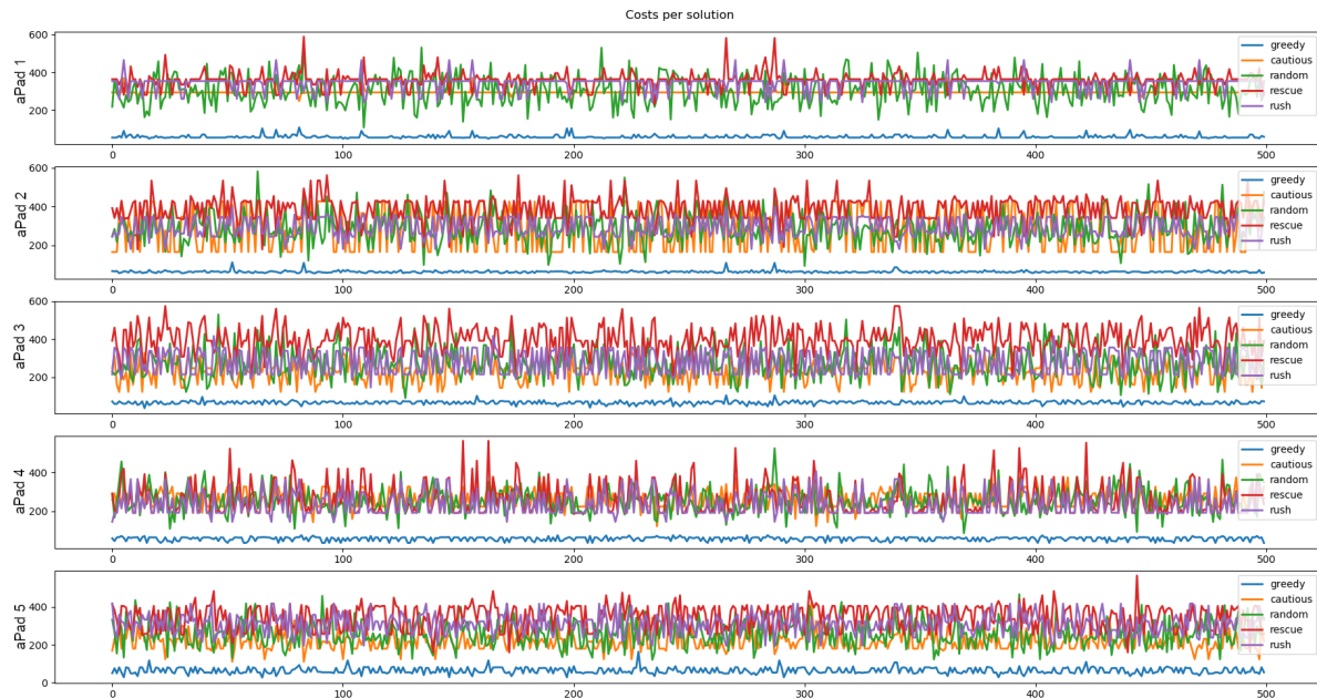
Figure 3.10: Distance cost plot for 500 experiment iterations performed on 5 aPads. Includes 120 aMussels and all 5 low-level heuristics.
