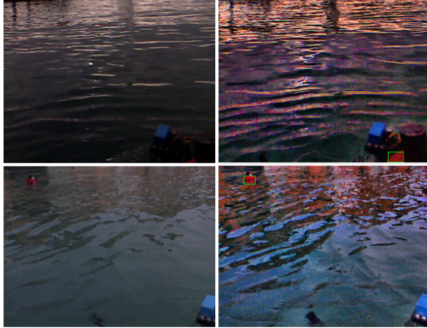
Figure 2.18: Two examples of aMussel cap detection - original images shown left and processed images shown right. The green rectangle on the camera image represents a bounding box around the derived position of the cap used to control the aPad's approach.
