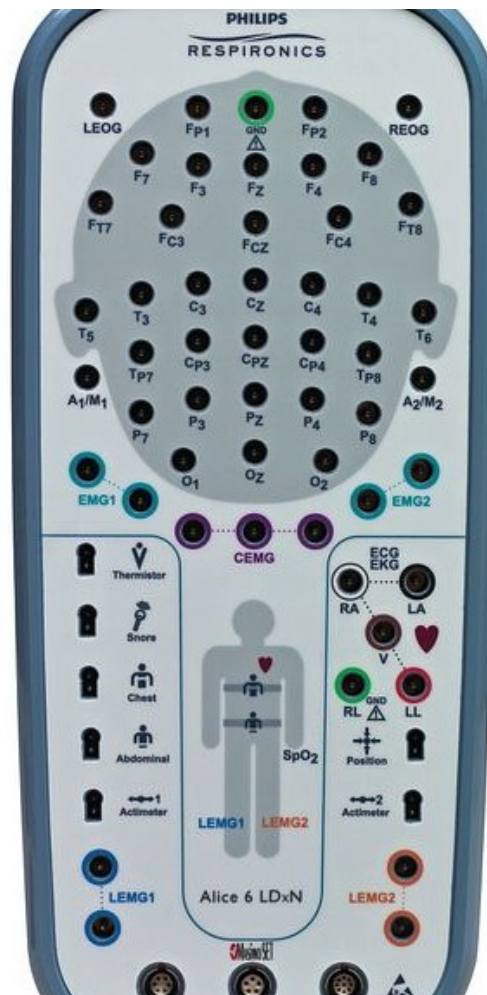
Figure 5.1 Alice 6 LDxN Philips Respironics PSG reference device [168]
